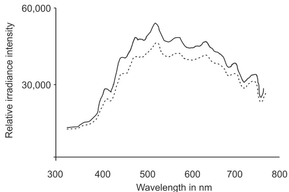
**Figure 4.** Measured relative irradiance of the natural sunlight spectrum compared to the light spectrum in the chamber.
