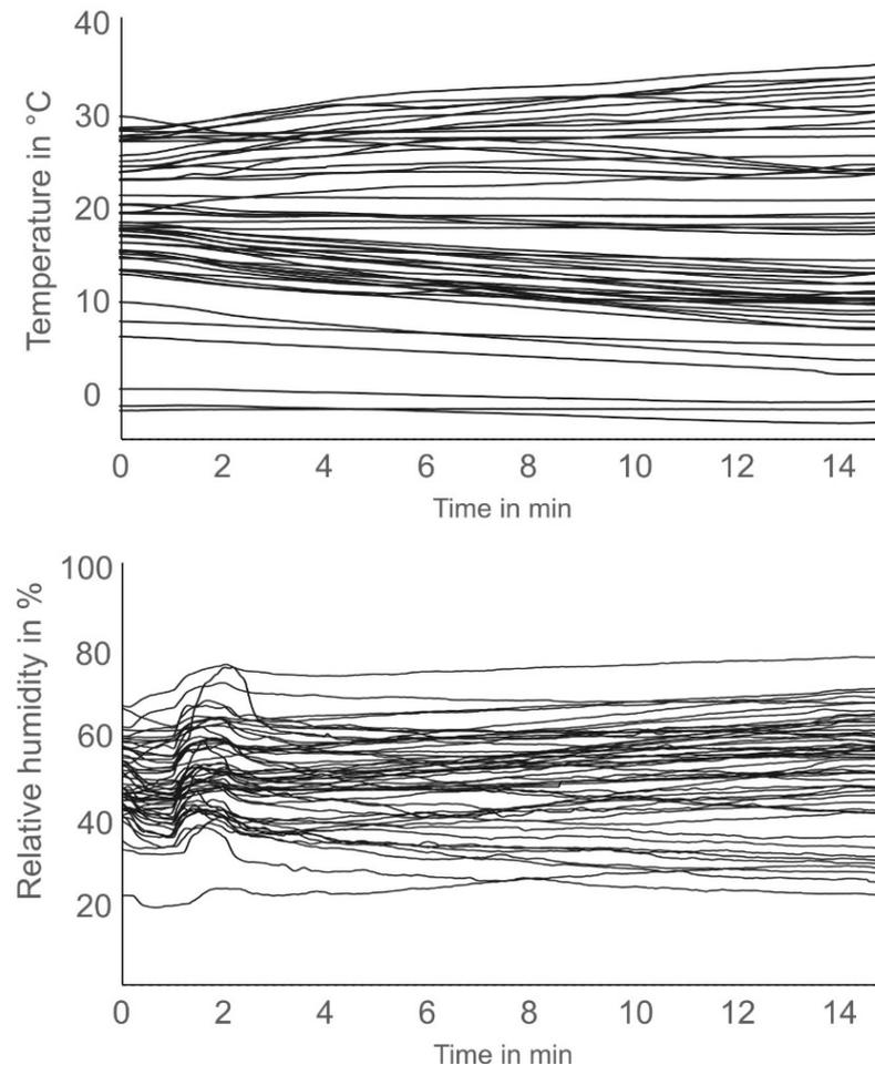
**Figure 3.** Course of temperature and relative humidity in the bioaerosol chamber during the 54 experiments.
