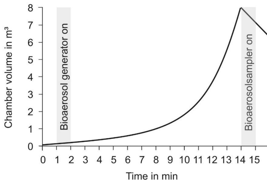
**Figure 2.** Schematic representation of the test procedure as a function of the chamber volume and the test time.
