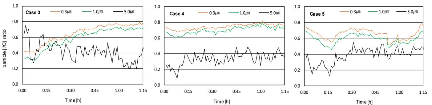
**Figure 7.** Particulate I/O ratio with a ventilation fan and natural ventilation (conditions 3–5).
