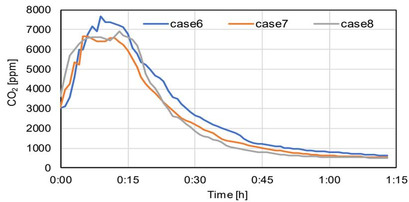
**Figure 5.** Carbon dioxide concentrations with use of a ventilation fan, natural ventilation, and an air conditioner (conditions 6–8).
