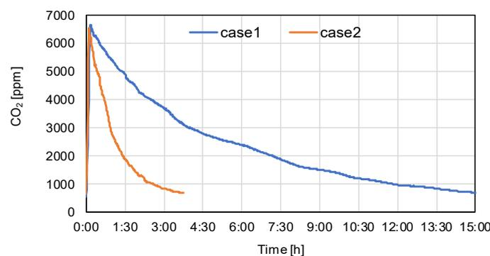
**Figure 3.** Carbon dioxide concentrations with and without a ventilation fan (conditions 1 and 2).
