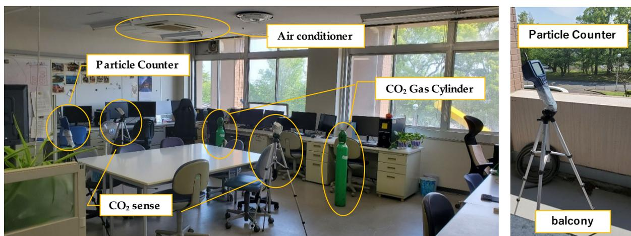
**Figure 2.** Indoor and outdoor measuring instruments.
