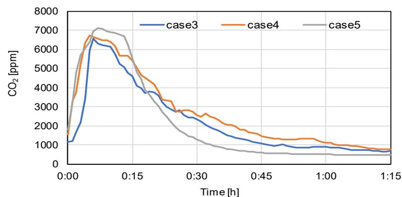
**Figure 4.** Carbon dioxide concentrations with a ventilation fan and natural ventilation (conditions 3–5).
