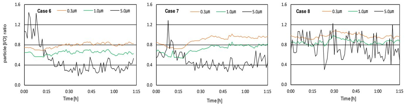
**Figure 8.** Particulate I/O ratios with a ventilation fan, natural ventilation, and an air conditioner (conditions 6–8).
