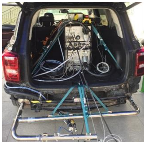
Figure 2. PEMS equipment installation diagram.
