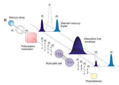
**Figure 1.** Lay-out of the Zeeman modulation correlation spectrometer (Lumex RA-915M; Courtesy: OhioLumex Corp., Cleveland, OH, USA).
