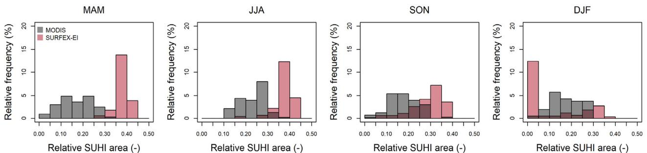
**Figure 5.** Histogram of relative SUHI affected area (compared to the total domain) at nighttime (top) and daytime (bottom) in each season in 2003–2005 over the city of Budapest.
