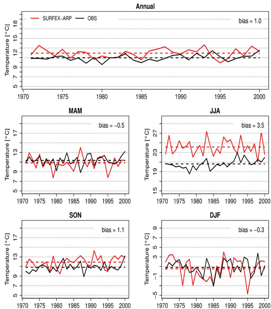
Figure 8. Annual and seasonal 2 m temperature ( $^{\circ}\text{C}$ ) of SURFEX-ARP in the suburban gridpoint and of the suburban station (Pestszentlőrinc) between 1971 and 2000. The 30 year average is marked with dashed lines and the mean bias indicated in the upper right corner.
