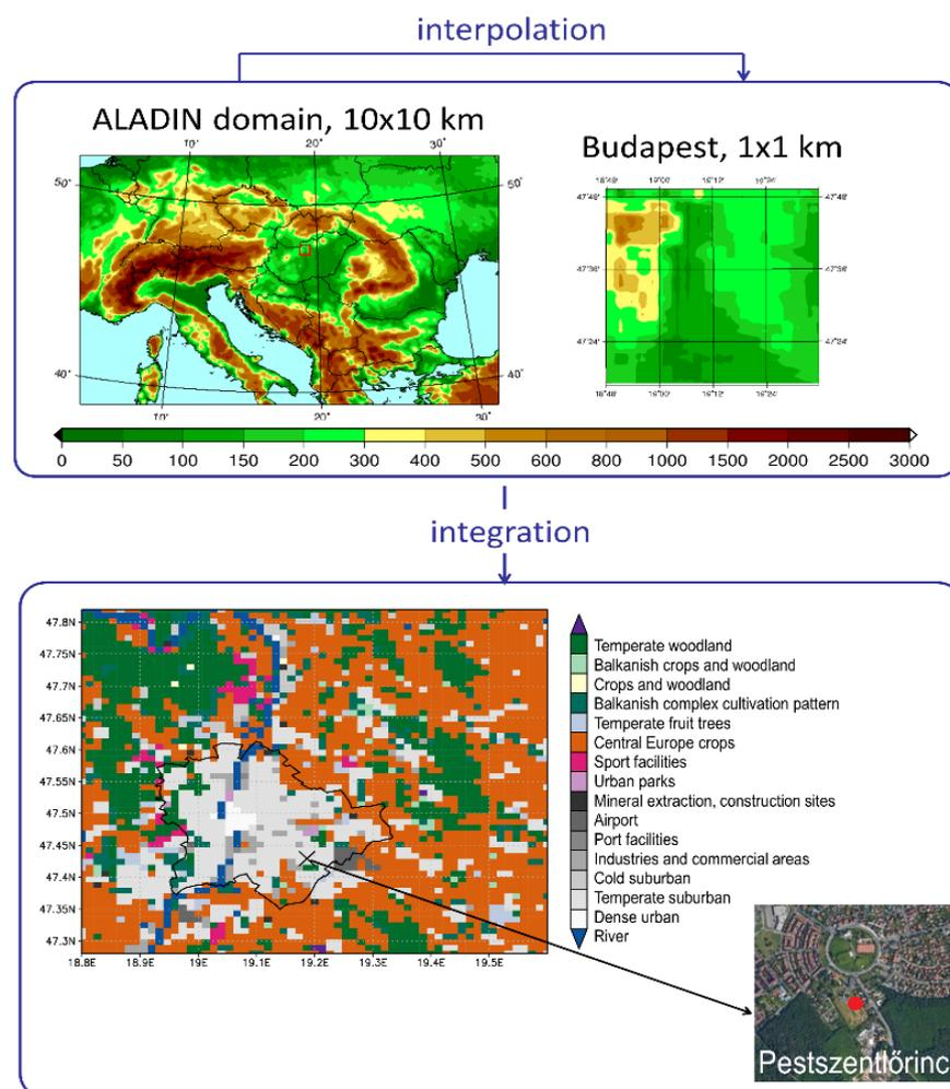
**Figure 1.** Flow chart about the use of SURFEX. Upper panel: domain and orography of the 10 km resolution ALADIN-Climate and its selected part covering Budapest, for which model fields are interpolated to 1 km resolution. Lower panel: land cover types according to the ECOCLIMAP database for the Budapest domain. Black X marks the closest gridpoint to the considered station measurement, which is also shown on orthophoto on the lower left corner (Google Earth image).
