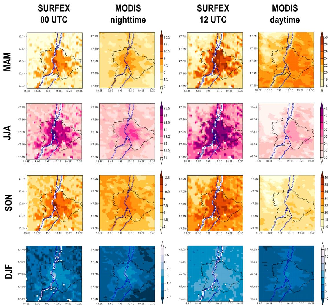
**Figure 3.** Seasonal mean land surface temperature ( $^{\circ}\text{C}$ ) in MODIS and radiative temperature in ALAD-EI driven SURFEX at 00 and 12 UTC in 2003–2005. Surface temperature over the Danube is masked out in the SURFEX results.
