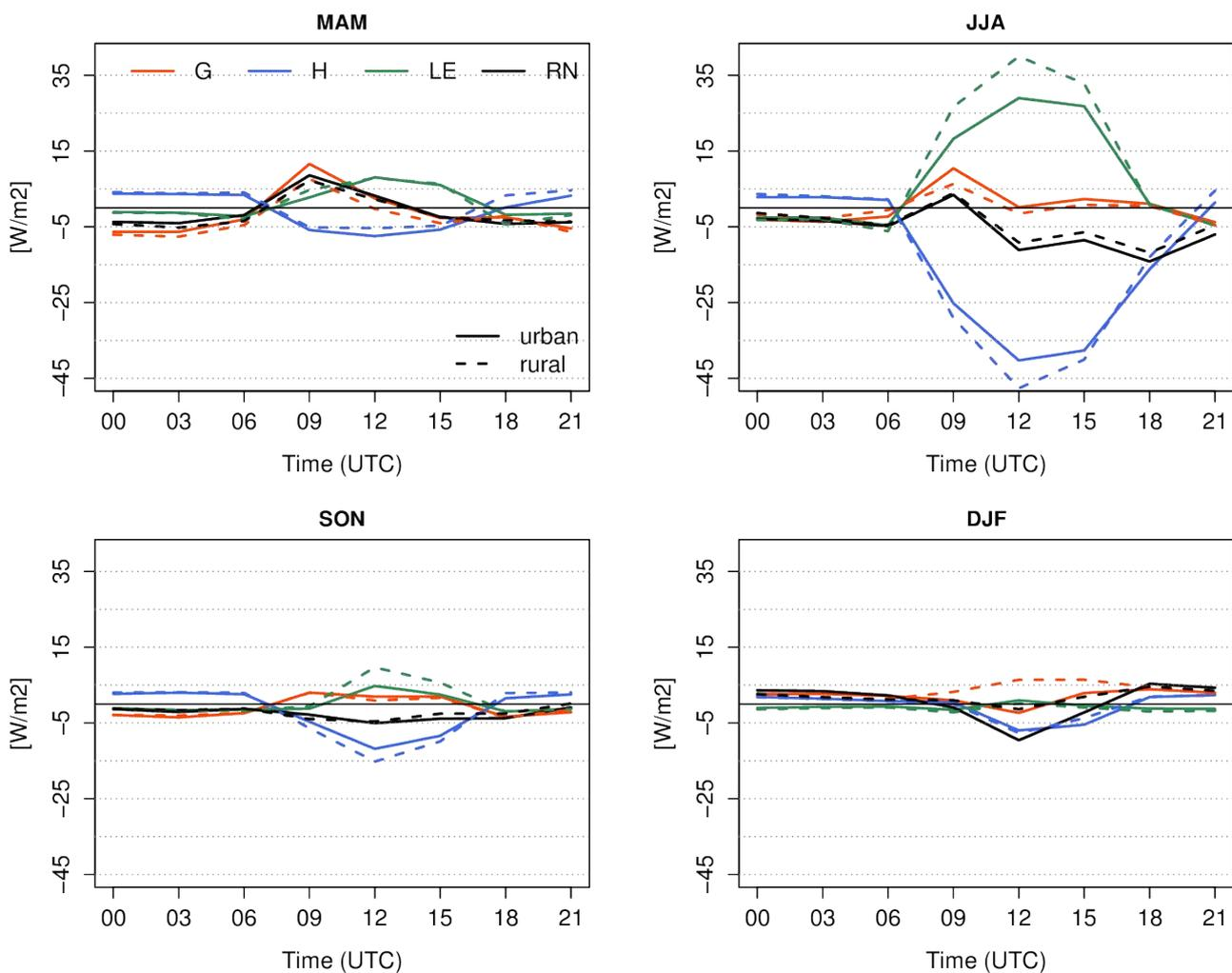
**Figure 12.** Difference ( $\text{W}/\text{m}^2$ ) of the seasonal mean diurnal cycle of surface energy budget components (RN: net radiation, H: sensible heat flux, LE: latent heat flux, G: ground heat flux) for the urban and rural grid points between the SURFEX-ARP and SURFEX-EI experiment. Period: 1996–2005.
