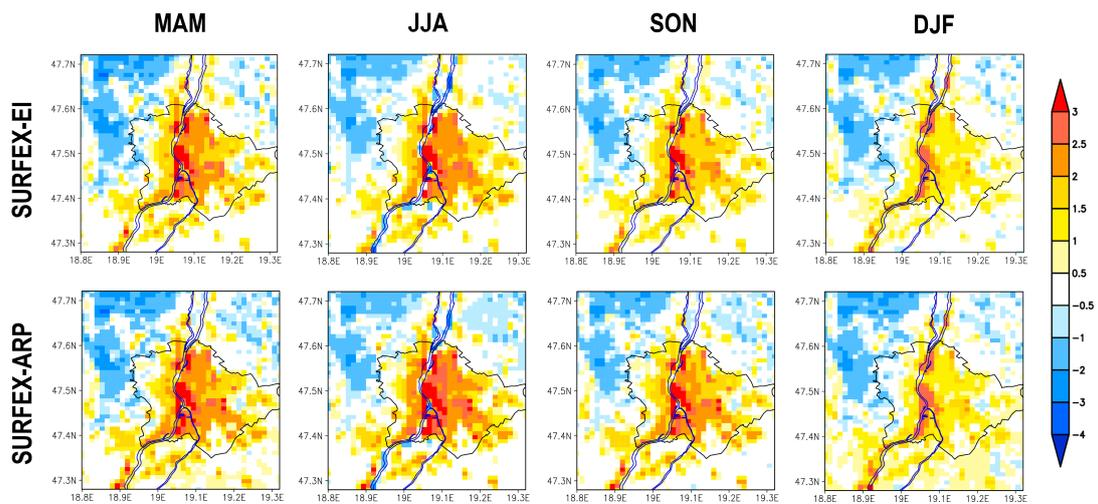
**Figure 11.** Seasonal mean urban heat island intensity ( $^{\circ}\text{C}$ ) based on SURFEX-EI and SURFEX-ARP for the period of 1996–2005. The spatial averages of the urban gridpoints are indicated above the corresponding maps.
