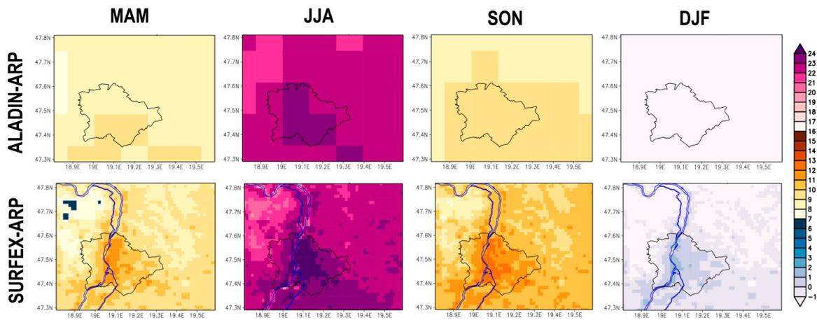
Figure 7. Seasonal mean 2 m temperature ( $^{\circ}\text{C}$ ) in ALADIN-ARP (first row) and SURFEX-ARP (second row) for the period of 1971–2000.
