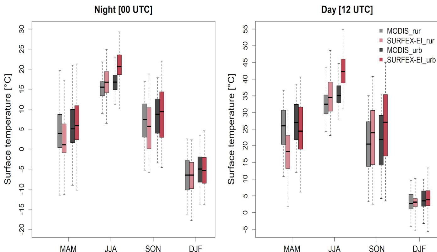
**Figure 4.** Box-whisker diagram of nighttime and daytime LST (°C) averaged over the urban and rural gridpoints in MODIS and SURFEX. Period: 2003–2005. The lower and upper boundaries of the boxes represent the lower and upper quartiles of the distribution, while the extent of the whiskers shows the minimum and maximum values. The median is represented by horizontal lines inside the boxes.
