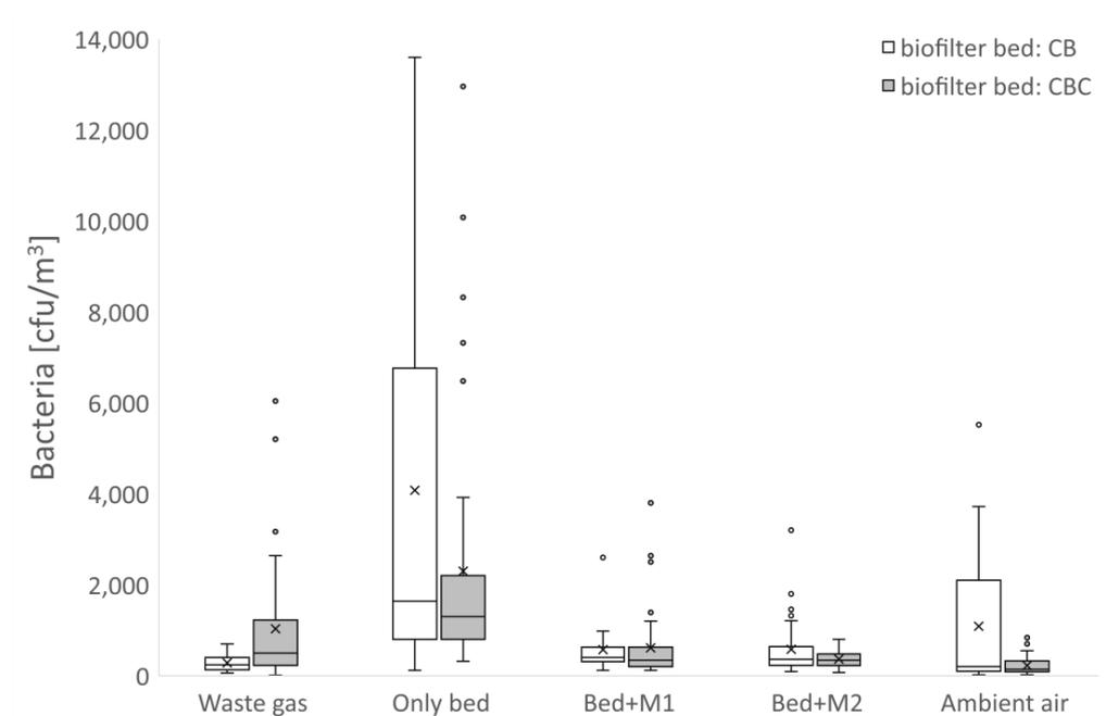
**Figure 3.** Total number of bacteria [cfu/m<sup>3</sup>] in the waste gas, gases treated by a conventional biofilter (only bed) and combined biofilter (bed + membrane M1 or M2), and the ambient air. Types of bed materials: CB—mix of stumpwood chips and pine bark; CBC—mix of stumpwood chips, pine bark, and compost from green waste. The band inside the box—median; ×—mean value; ○—outliers.
