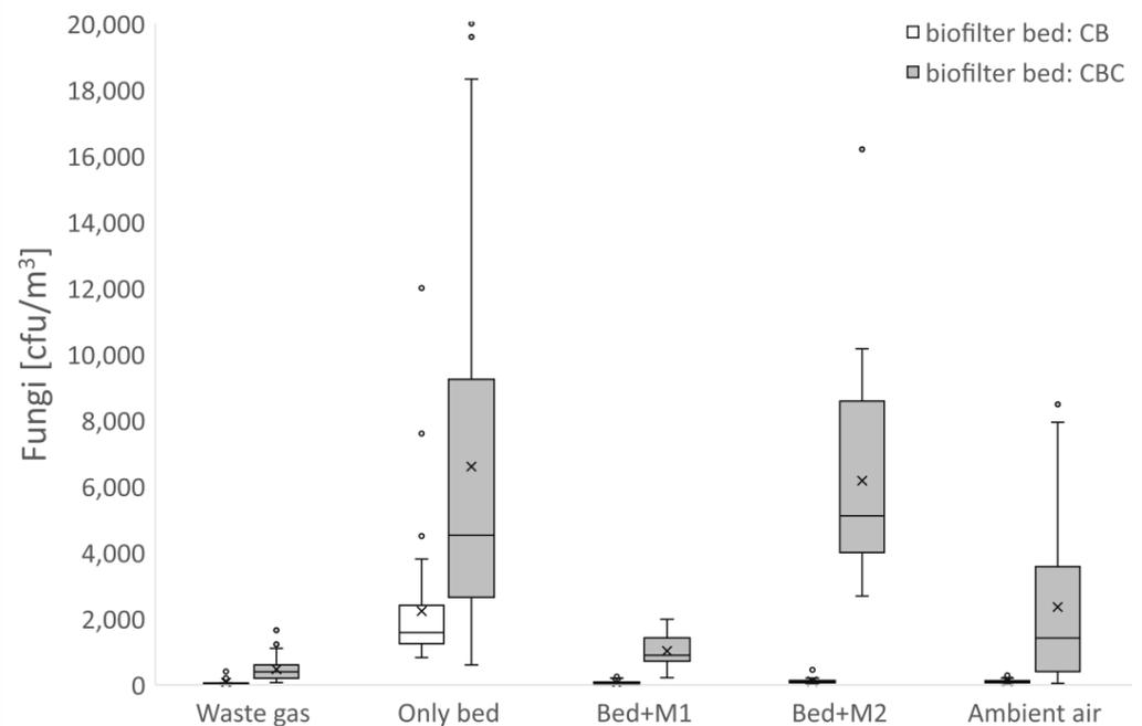
**Figure 4.** Total number of fungi [cfu/m<sup>3</sup>] in the waste gas, gases treated by a conventional biofilter (only bed) and combined biofilter (bed + membrane M1 or M2), and the ambient air. For a detailed legend, see Figure 3.
