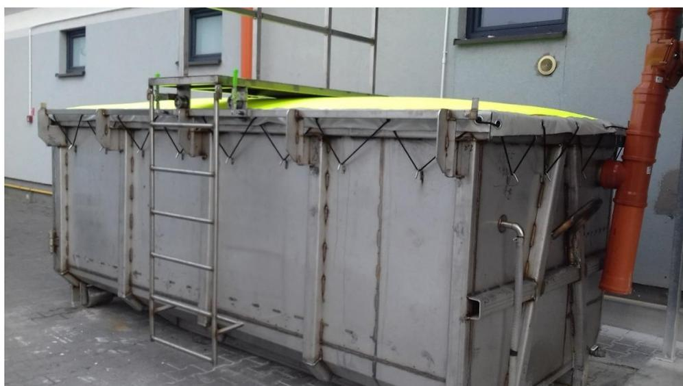
**Figure 2.** A pilot-scale combined biofilter examined for the treatment of waste gases from a food industry plant located in eastern Poland.
