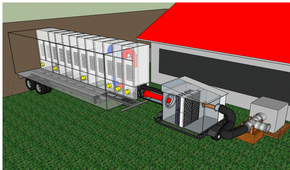
Figure 1. Schematic of a flow-through UV mobile laboratory with filtration unit connected to the continuous fan exhausting gas from stored manure headspace in the pit under barn’s slatted floor. The UV mobile lab consists of a series of connected chambers, each equipped with UV lamps (shown as panels of 5 in each chamber) and sprayed-on photocatalyst on surfaces (coated on all sides of the chamber except for the side installed UV). The lab treated up to 0.78 \text{ m}^3 \cdot \text{s}^{-1} of air. Excess airflow from the fan is discharged to the atmosphere. Cone-tipped ‘pipes’ signify free airflow inflow and outflow. Brown: exhaust air from swine barn; red: inlet air with reduced particle matter load; blue: UV-treated air. Yellow: gas sampling ports.
