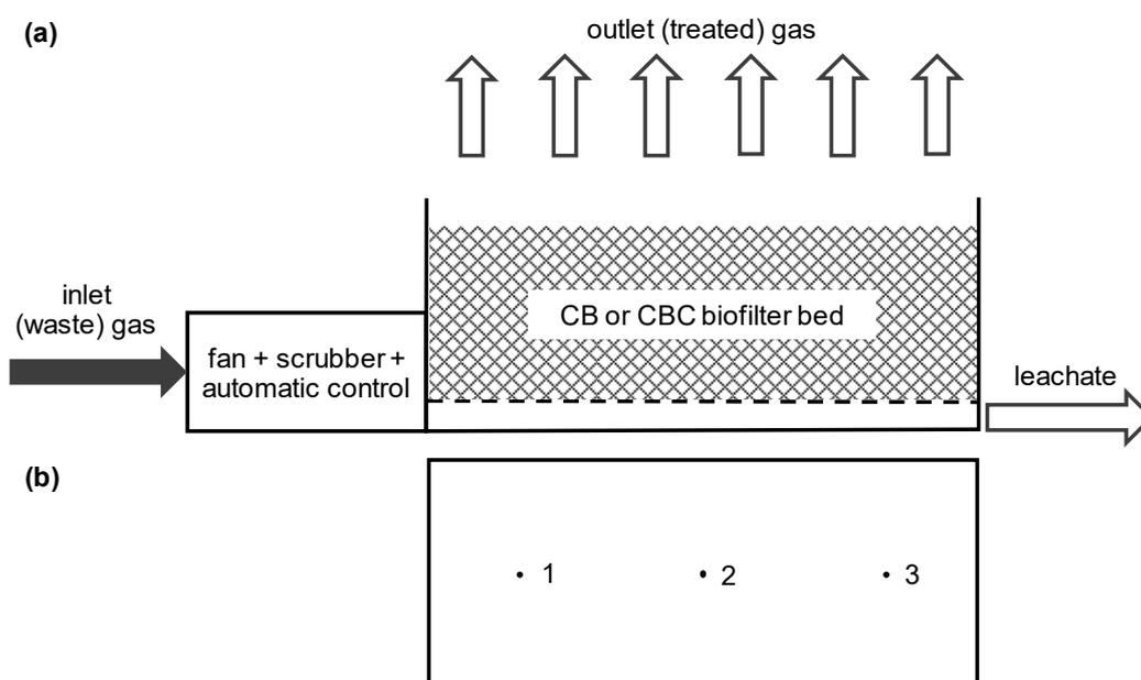
**Figure 1.** (a) Scheme of the pilot-scale biofilter equipped with a fan, a scrubber, an automatic regulation and control unit, and an installation for the distribution of waste gas and leachate drainage. Biofilter bed materials (CB—mix of stumpwood chips and pine bark; CBC—mix of stumpwood chips, pine bark and compost from green waste) were tested alternatively. (b) Location of sampling points (1, 2, 3) for bed material and treated gases—top view.
