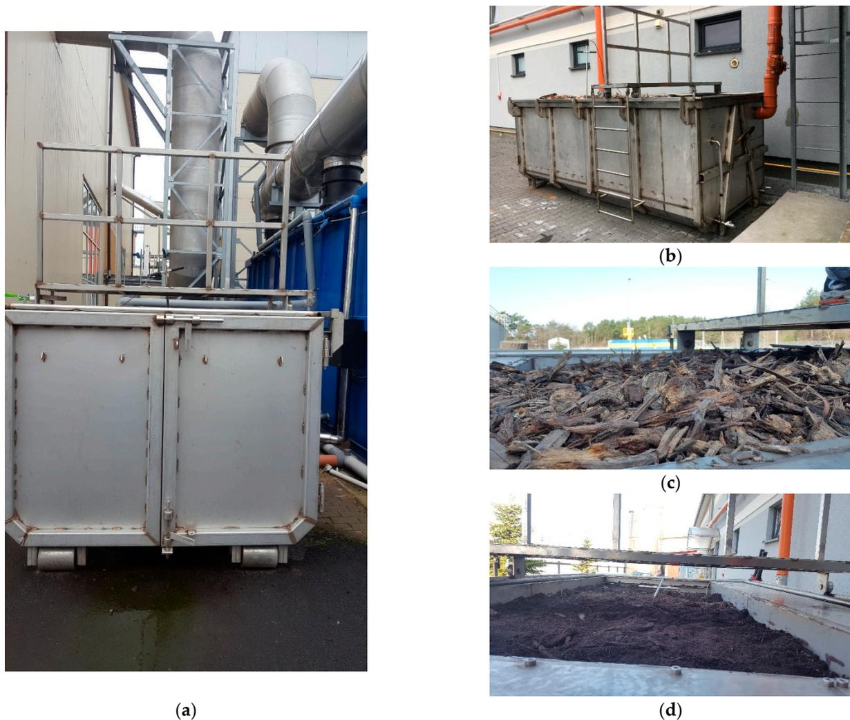
**Figure 2.** Pilot-scale biofilters tested for the treatment of waste gases from: (a) a wastewater treatment plant (WWTP) and (b) a food industry plant (FIP). (c) CB medium (mix of stumpwood chips and pine bark) in the pilot-scale biofilter tested for the treatment of waste gases from a mechanical–biological treatment plant (MBTP). (d) CBC medium (mix of stumpwood chips, pine bark and compost from green waste) in the pilot-scale biofilter at FIP.
