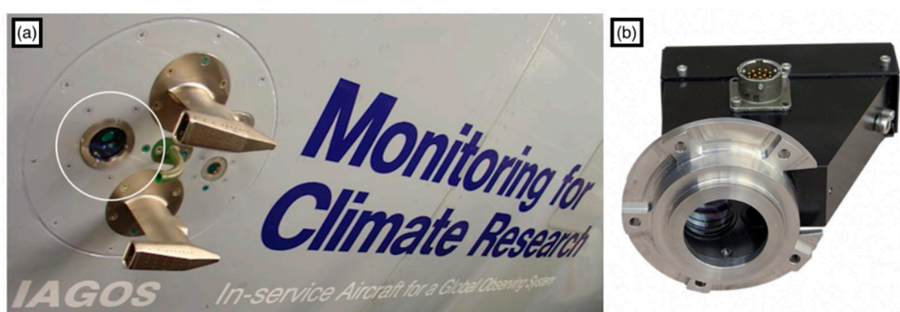
Figure 1. (a) Instrument installation on the In-Service Aircraft for a Global Observing System (IAGOS) instrumented Airbus and (b) the backscatter cloud probe (BCP).
