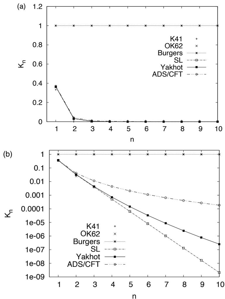
**Figure 2.** (a) reduced Kramers–Moyal coefficients from Equation (17) for different phenomenological models of turbulence up to the order  $n = 10$ . Coefficients for  $n > 2$  seem to tend towards zero; (b) semi-logarithmic plot of the reduced Kramers–Moyal coefficients. All phenomenological models except for K41 and OK62 show an asymptotic behavior. Note that the She–Leveque model possesses a nearly linear slope in the semi-logarithmic representation.
