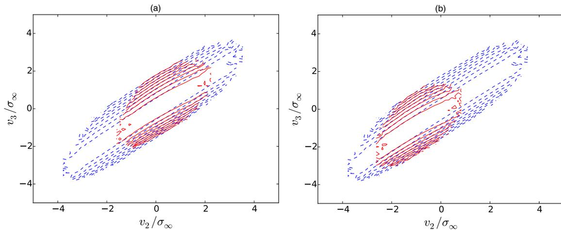
**Figure 21.** (a) examination of the Markov property (28) from DNS of the intermediate case for  $\Delta r = 2.2\lambda$  and  $v_1 = 0$  via a logarithmic contour plot. (b) same as in (a), but for  $v_1 = -\sigma_\infty$ . The shape of the conditional PDF (red) does not change significantly in comparison to (a).
