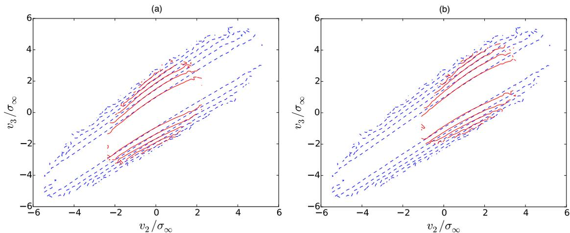
**Figure 14.** (a) examination of the Markov property (28) from DNS of the nonlocal case for  $\Delta r = 2.2\lambda$  and  $v_1 = 0$  via a logarithmic contour plot. (b) same as in (a), but for  $v_1 = \sigma_\infty$ . The shape of the conditional PDF (red) does not change significantly in comparison to (a).
