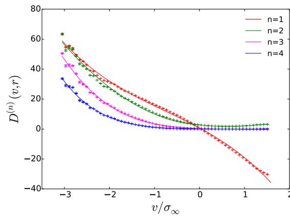
**Figure 11.** Estimation of the Kramers–Moyal coefficients from DNS of Burgers turbulence for  $r = L/2$ . The fits correspond to polynomials of the order  $n$  of the coefficient except for  $n = 1$  where a polynomial of order three has been used. The reduced Kramers–Moyal coefficients have been determined according to  $K_1 = 1.1689 \pm 0.08$ ,  $K_2 = 0.7880 \pm 0.14$ ,  $K_3 = 0.6956 \pm 0.17$  and  $K_4 = 0.7137 \pm 0.12$
