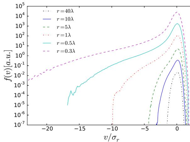
**Figure 5.** Evolution of the velocity increment PDF in scale (multiples of the Taylor length  $\lambda$ ) for the Burgers case  $\alpha = 1$ . The PDFs are shifted vertically and normed with their corresponding standard deviation  $\sigma_r$  for improved visualization. The pronounced left part of the PDFs is dominated by small-scale shock events, whereas the right part exhibits nearly self-similar behavior.
