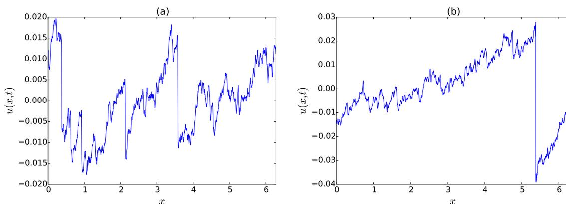
**Figure 3.** (a) typical realization of the velocity field  $u(x, t)$  in DNS of Burgers turbulence ( $\alpha = 1$  in Equation (26)). The velocity field exhibits a sawtooth profile that is due to the formation of large negative velocity gradients; (b) velocity field realization that belongs to the largest velocity gradient attained in the DNS belonging to Table 1.
