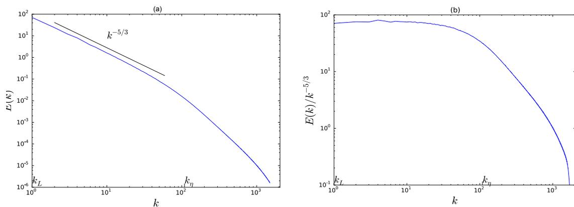
**Figure 13.** (a) energy spectrum  $E(k, t)$  of the velocity field of DNS of the nonlocal case. The inertial range obeys a Kolmogorov-like behavior  $\sim k^{-5/3}$ . (b) compensated energy spectrum  $E(k)/k^{-5/3}$ .
