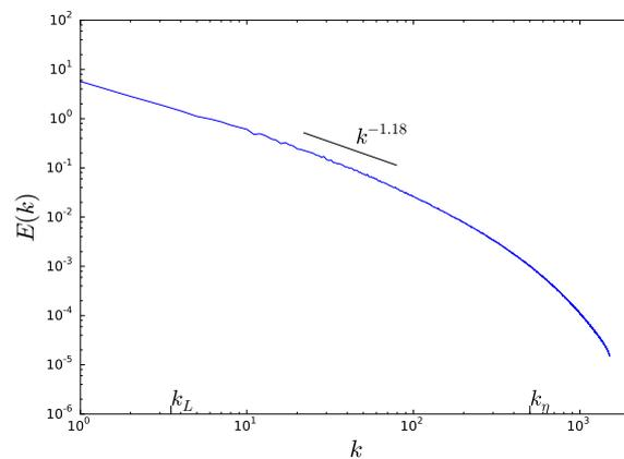
**Figure 20.** Energy spectrum  $E(k)$  from DNS of the intermediate regime ( $\alpha = 0.15$ ). The line indicates the spectral slope  $k^{-1.18}$ . No clear power-law behavior of the energy spectrum could be detected. The Kolmogorov spectrum might as well appear for larger  $k$  behind the indicated spectral slope.
