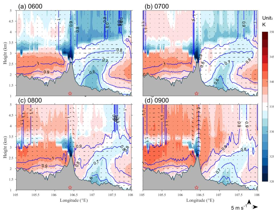
**Figure 6.** Cross-section of simulated pseudo-equivalent temperature (shaded, units: K) and specific humidity (blue solid lines, units:  $\text{g kg}^{-1}$ ) and wind field (black vectors, units:  $\text{m s}^{-1}$ ) along  $35.26^\circ \text{N}$ . (a) 0600, (b) 0700, (c) 0800, and (d) 0900 LST. The gray-shaded area is the terrain, and the red pentagram indicates the location of A1.
