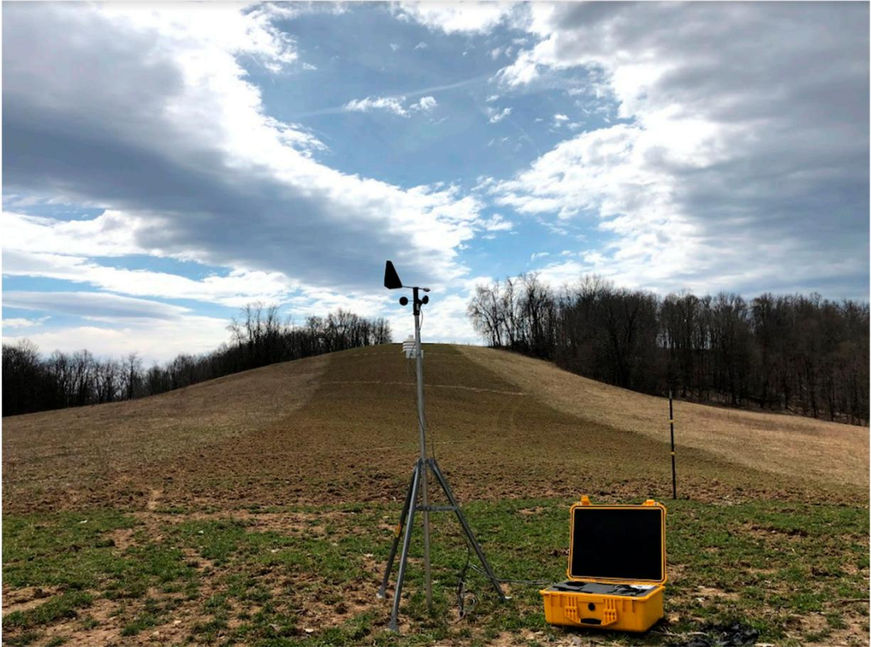
**Figure S2.** Portable weather station used to measure ground wind speed and direction.
