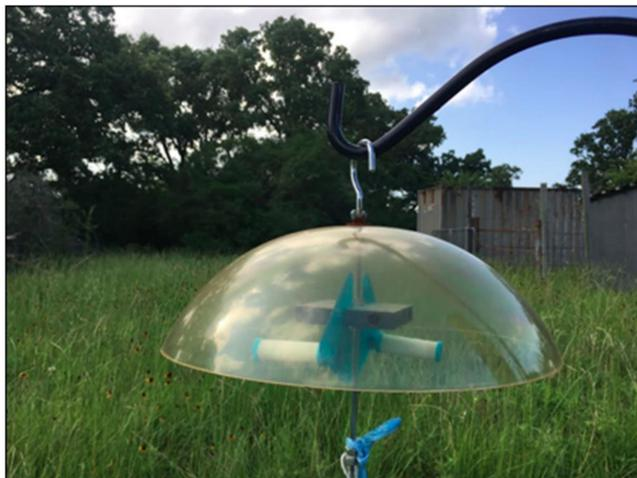
**Figure 1.** Sampling setup with Radiello diffusive bodies under the protective shelter.
