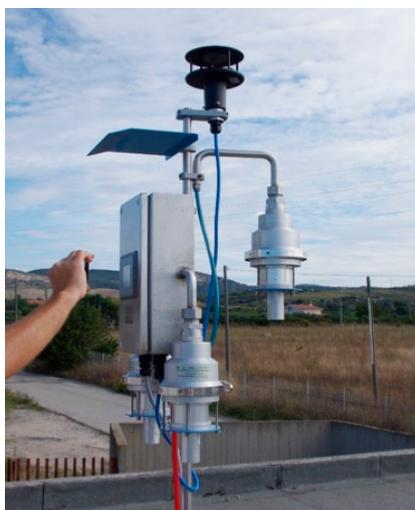
**Figure 1.** Wind-selective samplers used in this campaign.
