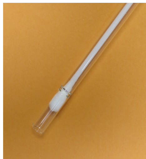
Figure 1. Swab inserted into glass Pasteur pipette. The tapered bottom of the apparatus was connected to a vacuum via plastic vacuum tubing. The cylindrical top containing the swab head was dragged across the paper surface to dry vacuum.
