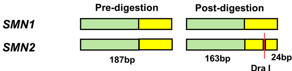
Figure 1. Primer positions and pre- and post-digestion products in PCR-RFLP analysis. Dra I treatment creates two products of 187 bp and 24 bp from SMN2 fragment, but it does not lead to any change in SMN1 fragment.
