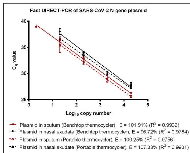
**Figure 2.** Fast DIRECT-PCR assay amplification efficiency of SARS-CoV-2 N gene plasmid spiked in sputum (red line) and N gene plasmid spiked in nasal exudate (black line) using the benchtop thermocycler (solid line) and the portable thermocycler (dotted line). Templates were ten-fold diluted in 6 orders of magnitude. One microliter of template was used in 10  $\mu$ L of PCR mastermix.
