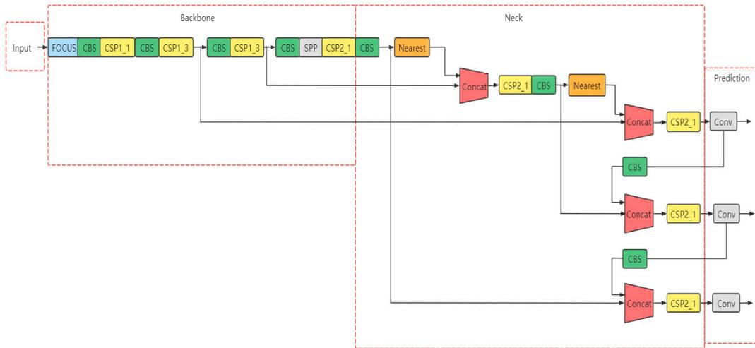
Figure 2. The architecture of the network of YOLOv5s in this paper.
