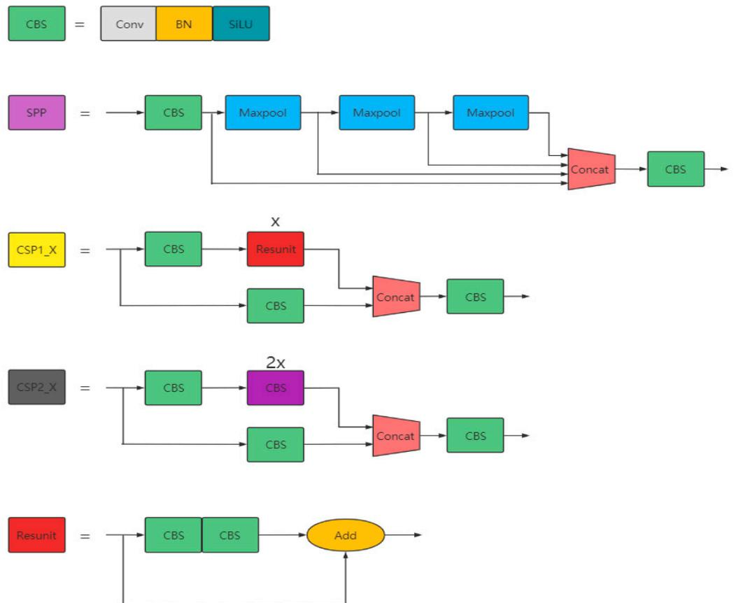
Figure 3. Composition of modules in YOLOv5s.
