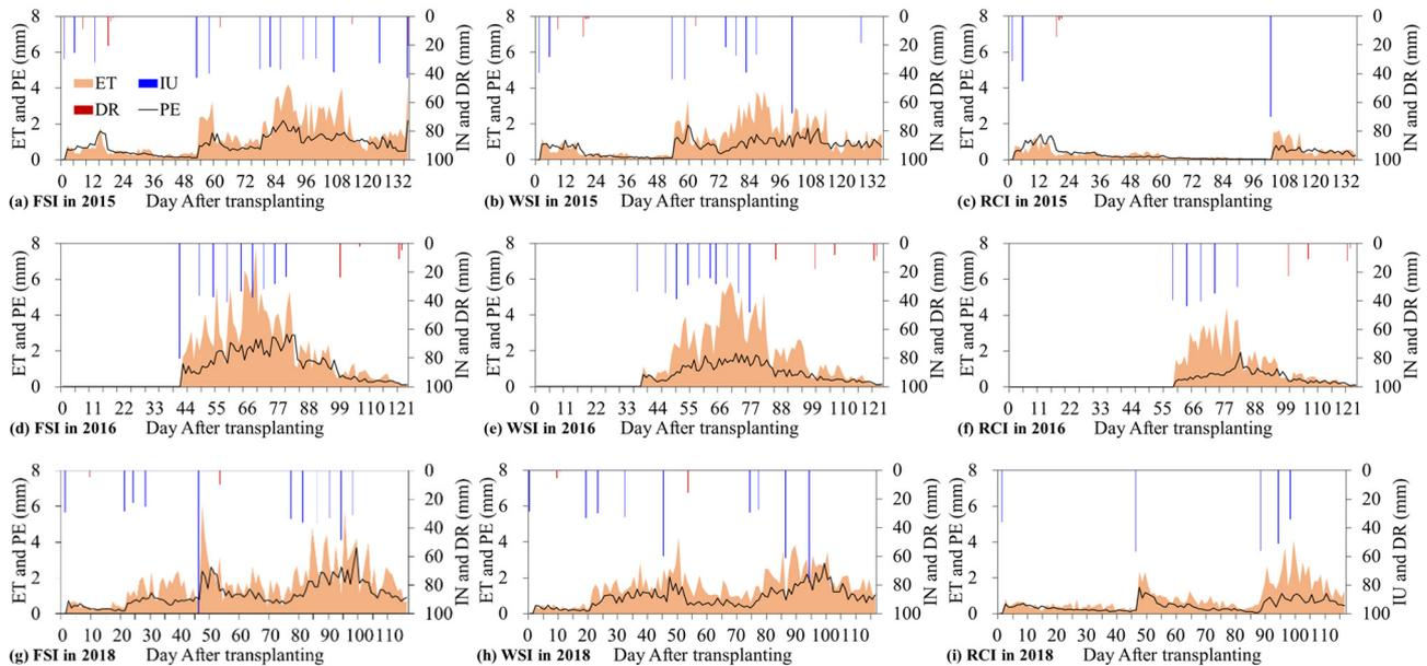
**Figure 2.** Daily blue water balance in for the three irrigation modes in the years 2015, 2016, and 2018. (IN: blue water inflow; ET: blue water evapotranspiration; PE: blue water percolation; DR: blue water drainage).
