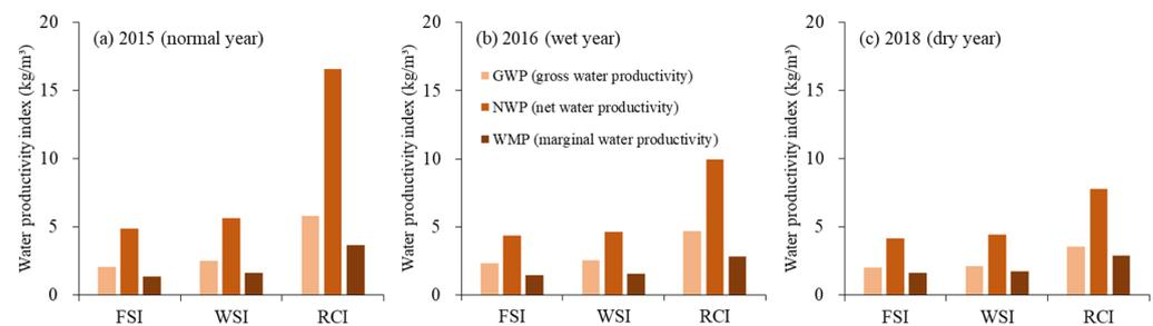
**Figure 4.** Irrigation water productivity indicators in paddy field in normal, wet, and dry years.
