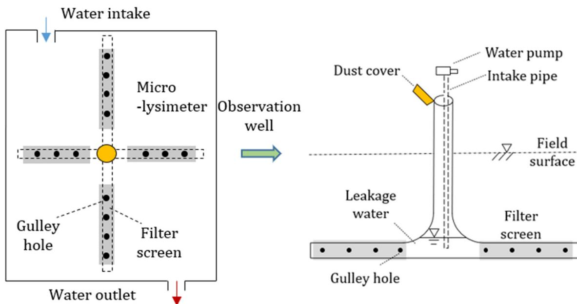
**Figure 1.** Arrangement diagram of field measurement.
