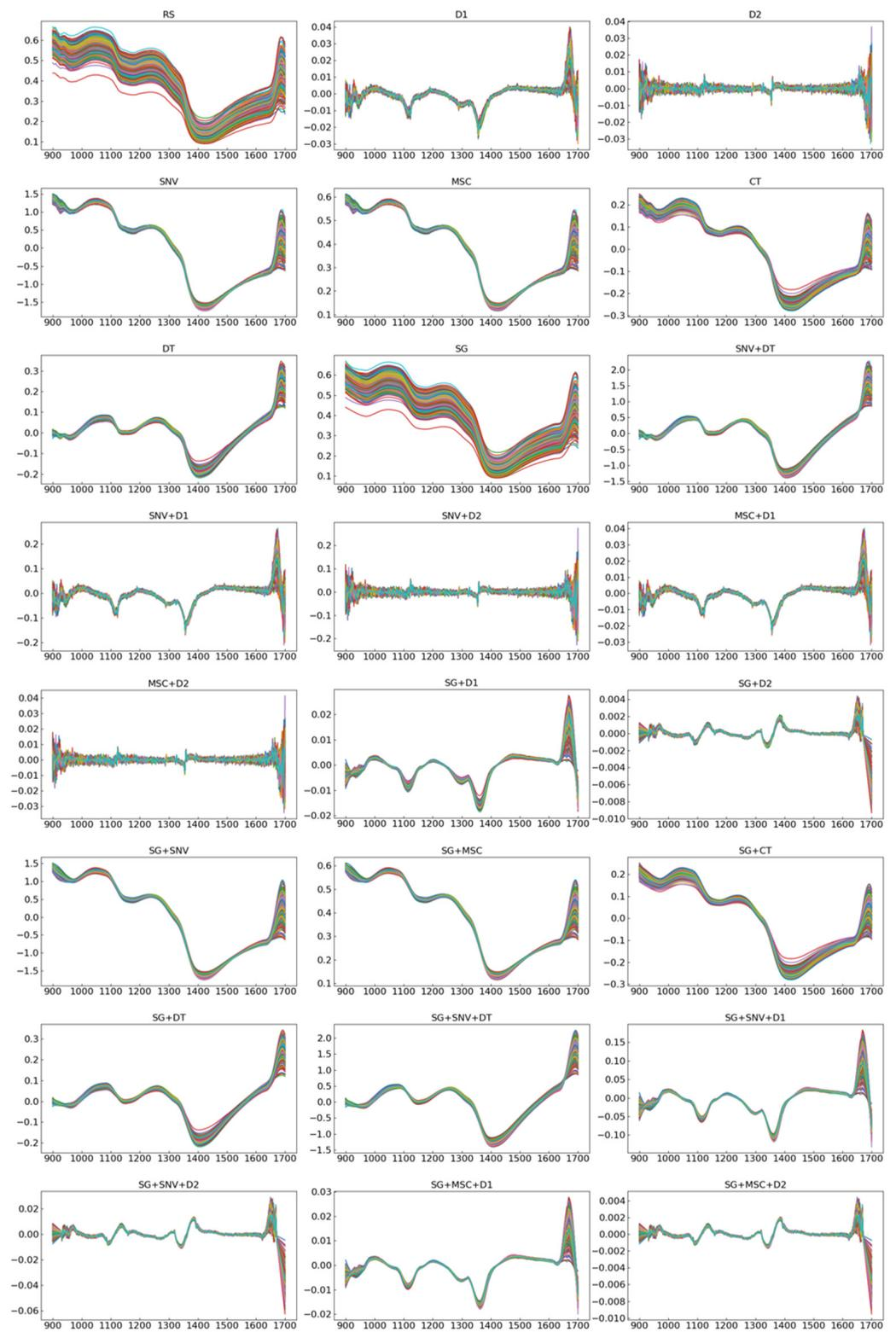
Figure 4. NIR spectra with different pretreatment transformations.
