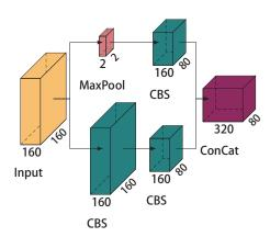
Figure A2. MPC3 Module.
