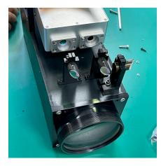
Figure 3. A handhold Raman Spectroscopy detection device.
