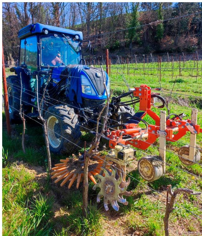
Figure 3. View of the tool-holder positioned in the tractor front area, and disposition of rollhackle and finger weeder.
