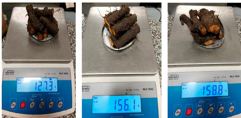
**Figure 2.** Weight the cut knotweed rhizomes before microwave treatment.
