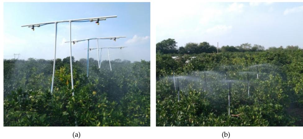
**Figure 3.** Spraying units of fixed spraying systems: (a) spraying unit equipped with pressure-swirl nozzles; (b) spraying unit equipped with fixed spray plate sprinklers.
