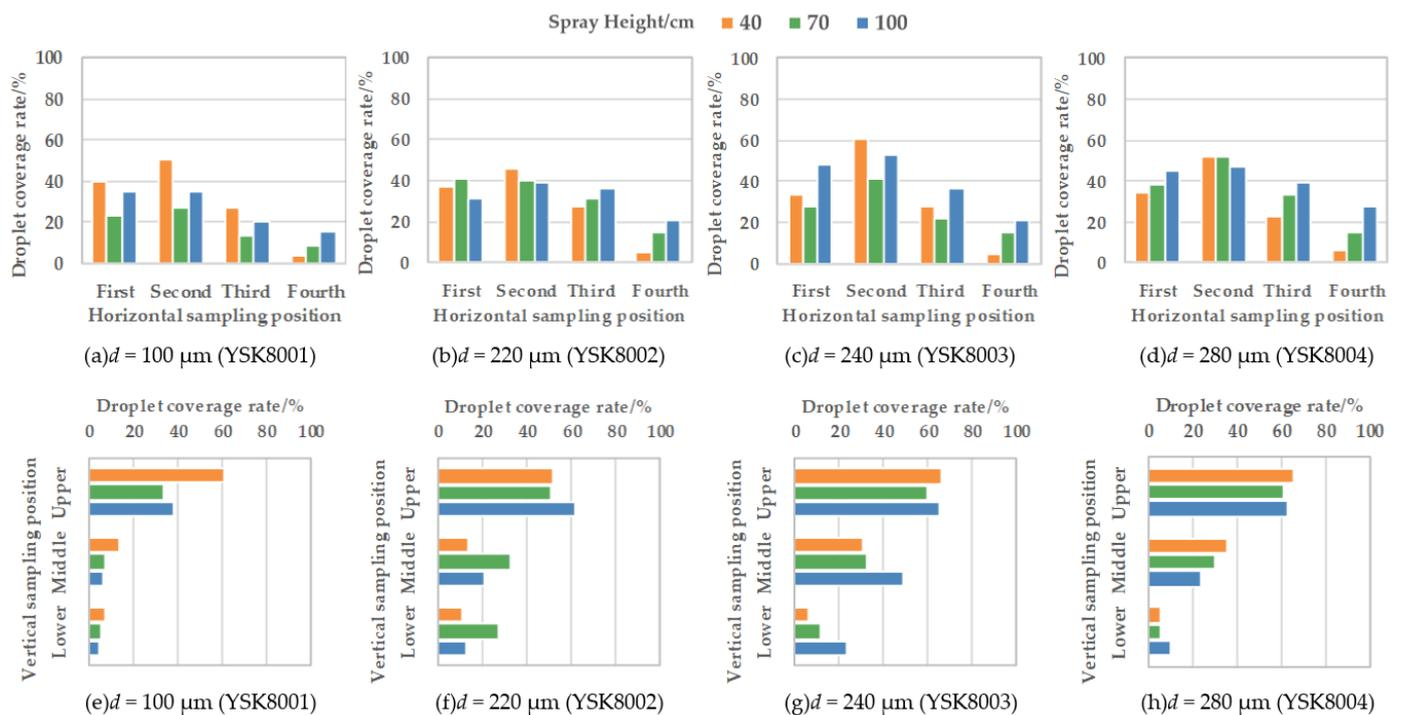
**Figure 5.** DCR of pressure-swirl nozzles in citrus canopy: (a–d) represent DCR in horizontal direction; (e–h) represent DCR in vertical direction.
