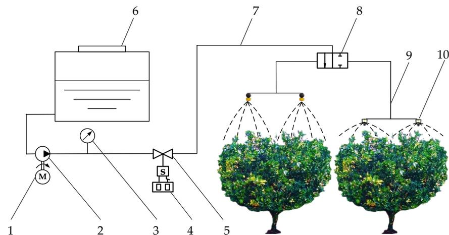
**Figure 1.** Fixed spraying system prototype: 1. Electro-motor; 2. Plunger pump; 3. Pressure gage; 4. Time relay; 5. Solenoid valve; 6. Tank; 7. Hose; 8. Distribution valve; 9. Support frame; 10. Nozzle.
