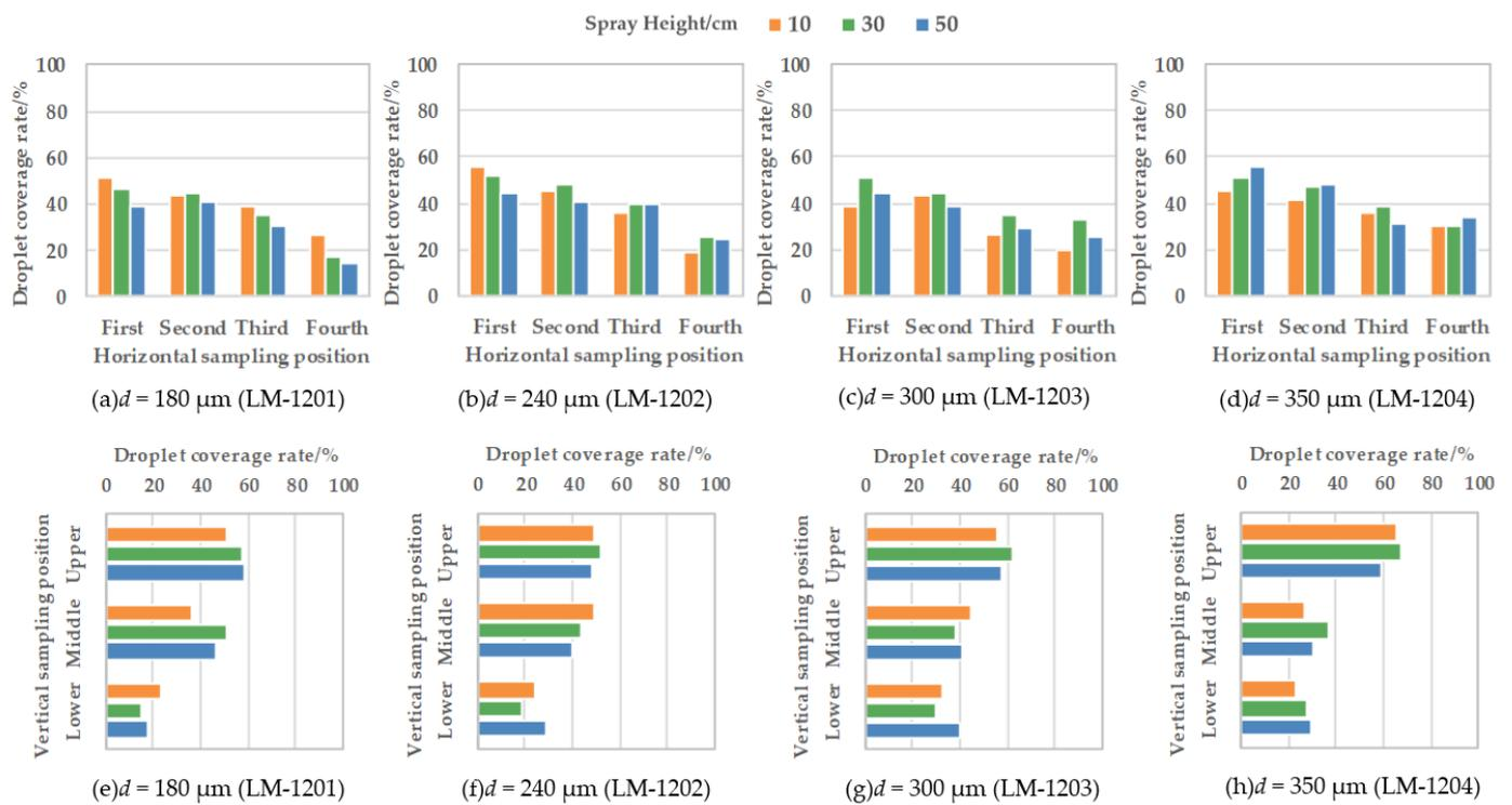
**Figure 6.** DCR of fixed spray plate sprinklers in citrus canopy: (a–d) represent DCR in horizontal direction; (e–h) represent DCR in vertical direction.
