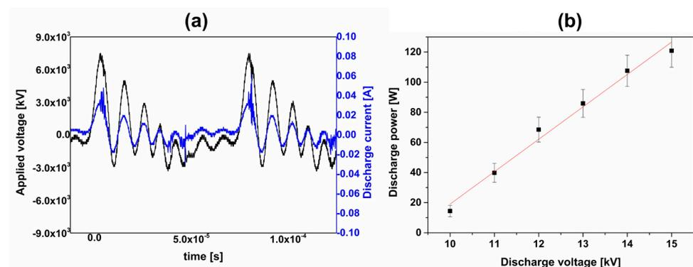
**Figure 2.** (a) Typical IV characteristic of the discharge and (b) estimation of the NTP power as a function of the peak-to-peak discharge voltage value from electrical measurements.
