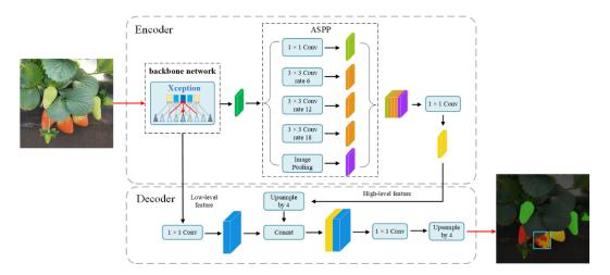
Figure 5. DeepLabV3+ structure and segmentation effect.
