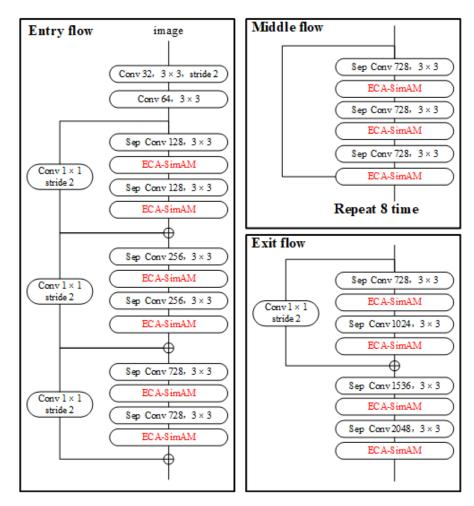
Figure 8. Dual-attention mechanism to optimize the backbone network.
