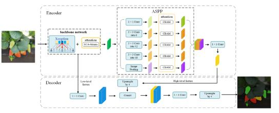
Figure 6. Improved DeepLabV3+ network structure diagram.
