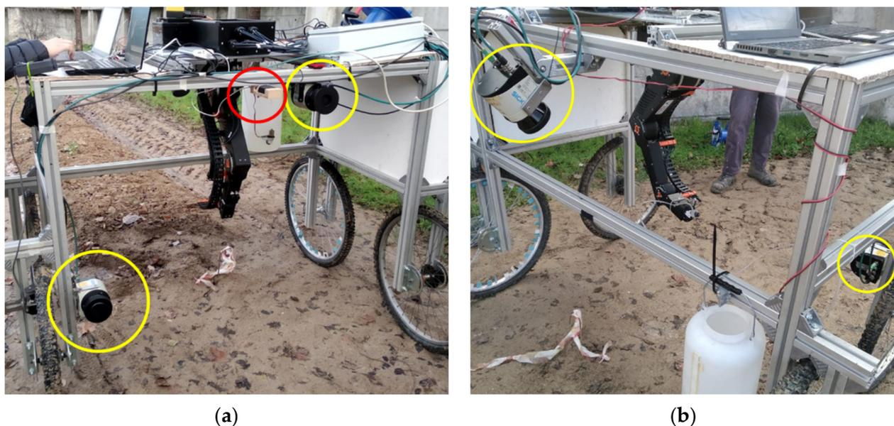
**Figure 1.** Frontal view (b) and rear of the platform (a), the yellow circles show the 3 LiDAR sensors and the red circle indicates the multispectral camera.
