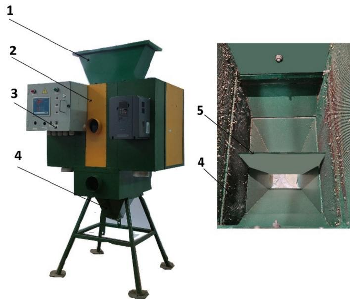
**Figure 11.** External view of a microwave-convective grain processing plant: (1) loading hopper; (2) microwave-convective processing unit; (3) control system unit; (4) unloading hopper; (5) bulk material flow separator.
