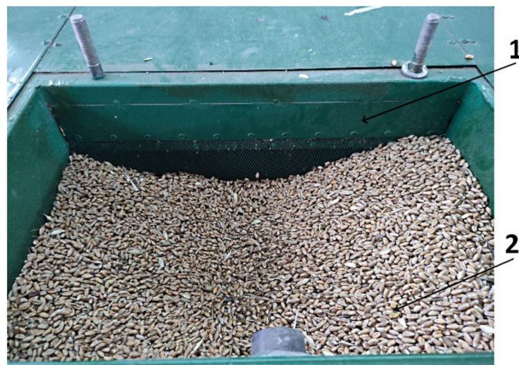
**Figure 12.** Grain in the microwave-convective zone within the experiment: (1) active zone for microwave-convective grain processing; (2) grain in the microwave-convective zone.
