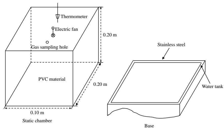
**Figure 2.** Static chamber.
