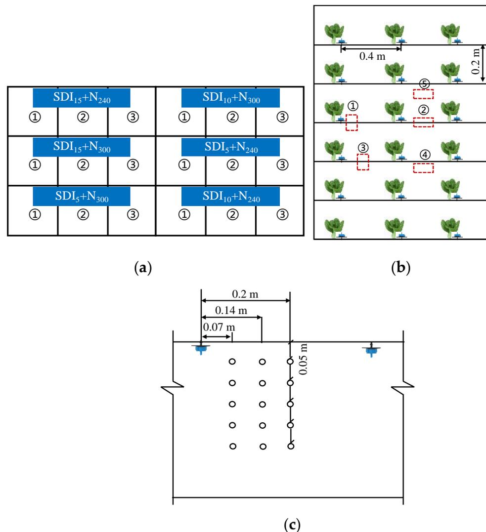
**Figure 1.** Experimental layout of subsurface drip irrigation system. Treatment layout (a), plot layout (b), and horizontal distances from the dripper point (c).
