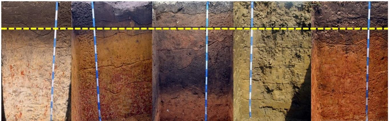
**Figure 6.** Photographs of five soil profiles of the study area indicating the topsoil (30 cm). The horizontal-yellow line indicates the “arable layer of the soil”; The vertical line with alternating colors every 10 cm is the tape measure.
