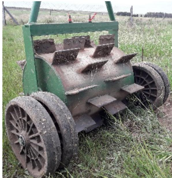
**Figure 2.** Roller-crimper.
