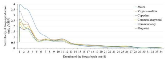
**Figure 3.** Net velocity of biogas production per gram volatile solids from the crops tested in this study. For each measurement and for each crop except mugwort, the error bars indicate the standard deviation for the replicates of the crop species in the field trial.
