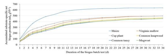
**Figure 4.** Accumulated substrate-specific net biogas production of the crops investigated in this study. For each measurement and for each crop except mugwort, the error bars indicate the standard deviation for the replicates of the crop species in the field trial.
