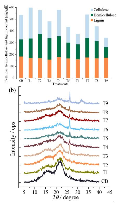
**Figure 4.** The contents of cellulose, hemicellulose, and lignin (**a**) and the x-ray diffractions (**b**) of the remaining chestnut burrs (CB) at the end of composting (CB: initial chestnut burrs, T1–T9: the remaining CB in treatments T1–T9).
