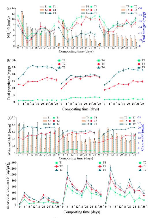
**Figure 2.** Temporal variation in  $NH_4^+$ –N content and total Kjeldahl nitrogen content (**a**), water-soluble P and citric acid-P (**c**) during the composting process (bar diagram is represented by primary *y*-axis and line diagram by secondary *y*-axis (blue)). Variation in total phosphorus content (**b**) and microbial biomass P (**d**) during the composting process. Treatments T1–T9 are described in Table 1.
