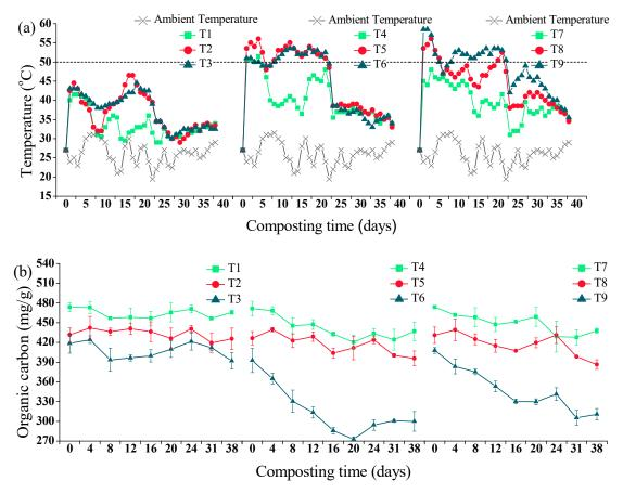
**Figure 1.** Variation in composting temperature (**a**) and organic carbon content (**b**) during the composting process. Treatments T1–T9 are described in Table 1. The part above the dotted line in (**a**) represents the time of the thermophilic period during composting.
