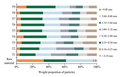
**Figure 5.** Variation in particle size distribution of the initial CB and final products (Raw material: initial CB, Treatments T1–T9 are described in Table 1).
