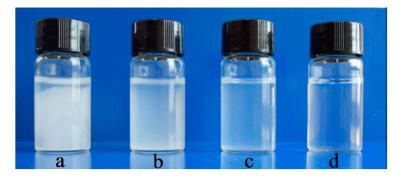
**Figure 5.** Dispersion states of (**a**) pristine cellulose; (**b**) NaOH/urea-treated cellulose; (**c**) direct TEMPO-oxidized cellulose; and (**d**) NaOH/urea-treated TEMPO-oxidized cellulose.
