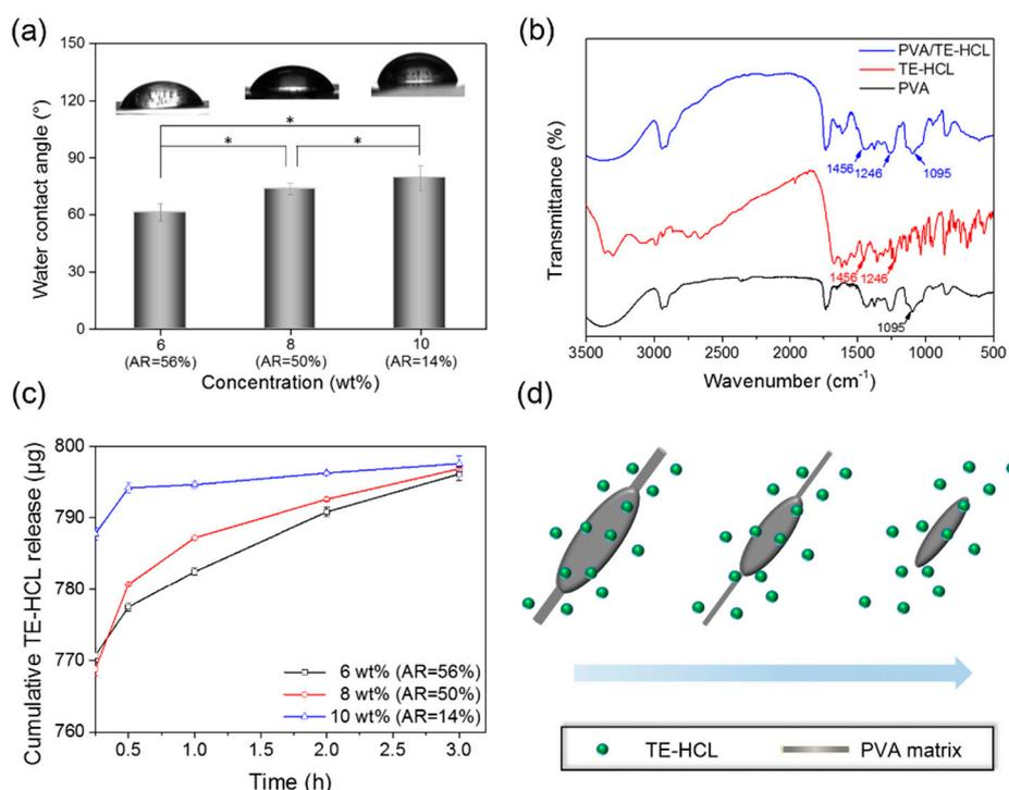
**Figure 5.** (a) Water contact angles on PVA fibrous membranes prepared using 6, 8, and 12 wt % PVA solutions (bead fiber AR = 14%, 50%, and 56%, respectively). (b) FTIR spectra of neat materials and samples prepared in this study. (c) TE-HCL release profiles from PVA matrices prepared using various solution concentrations. (d) Schematic illustration of drug release from PVA beaded fibers over time (\*  $p < 0.05$ ).
