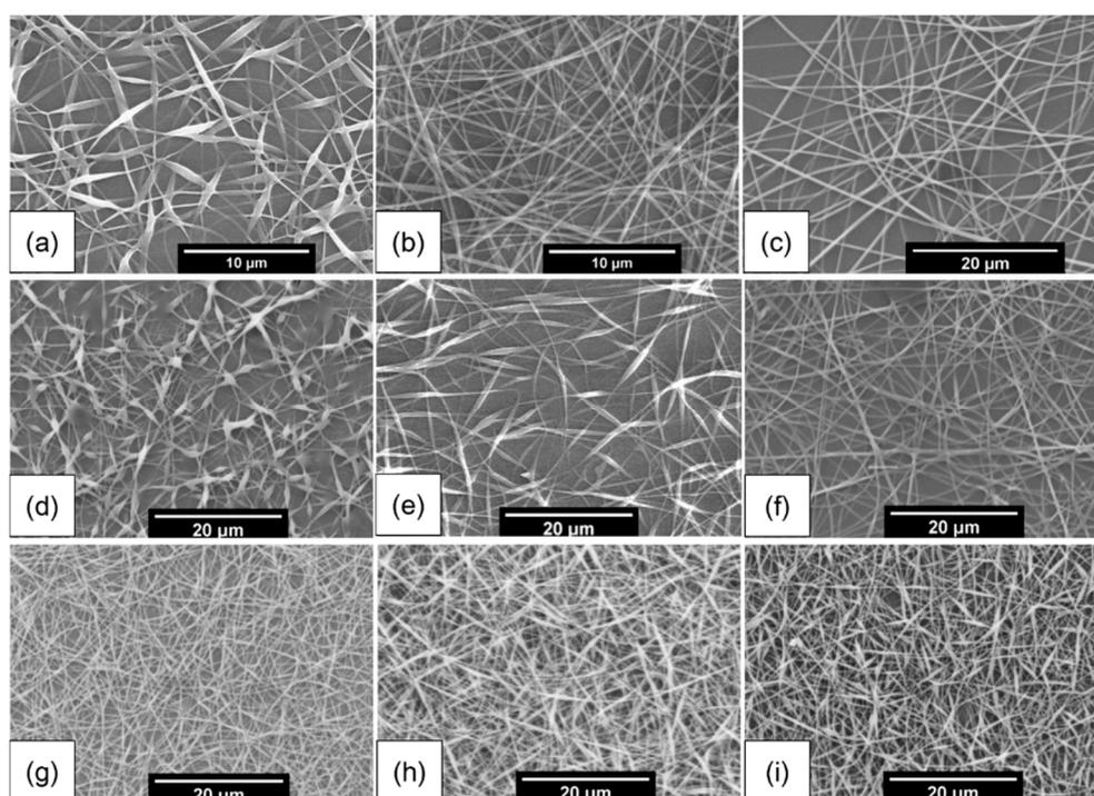
**Figure 3.** Scanning electron micrographs. Nanofibers produced using various pure PVA solutions (parameters 60 °C, 100 rpm for 60 min; all other conditions are constant): (a) 6; (b) 8; and (c) 10 wt %. Nanofibers produced using various PVA microbubble suspensions (all other parameters constant): (d) 6; (e) 8; and (f) 10 wt %. Nanofibers prepared using PVA microbubble suspensions and various applied voltages (all other parameters constant): (g) 14; (h) 16; and (i) 18 kV.
