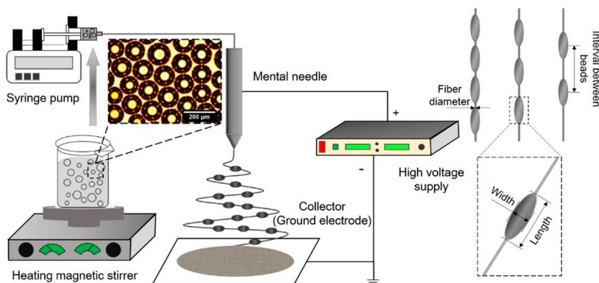
**Figure 1.** Schematic diagram of an electrospinning (ES) apparatus for beaded fiber engineering and graphical illustration of the key fiber properties assessed in this study.
