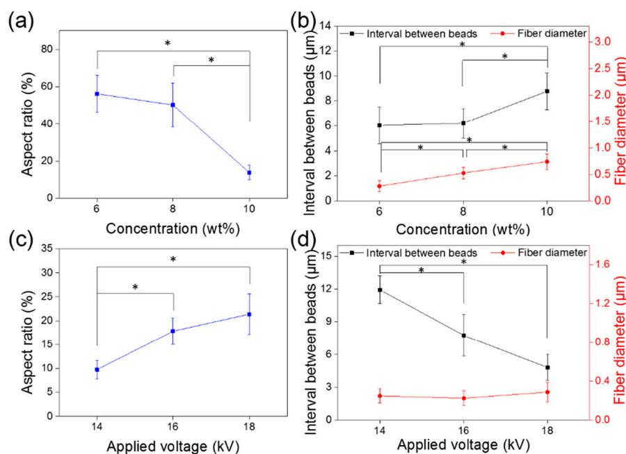
**Figure 4.** Effect of solution concentration on fiber properties: (a) bead AR; (b) inter-bead distance. Effect of applied voltage on fiber properties: (c) bead AR; (d) inter-bead distance. (\*  $p < 0.05$ ).
