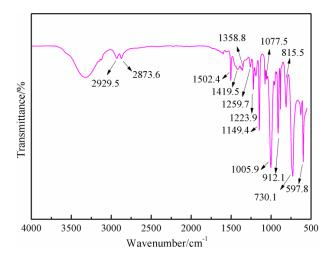
Figure 7. FT-IR spectrum of furfuryl alcohol (FA).
