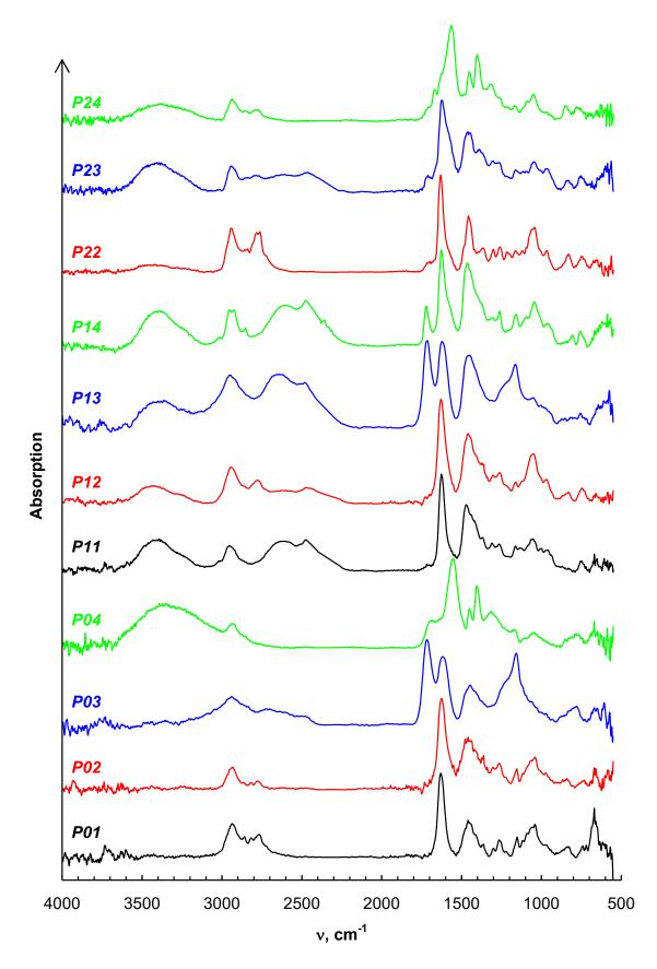
Figure S1. FTIR spectra of the new polymers. The CO<sub>2</sub> band at 2300 cm<sup>-1</sup> was erased.
