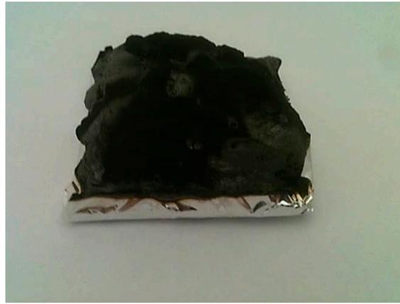
**Figure 8.** Residue of H/E-15APP after cone calorimetry tests.
