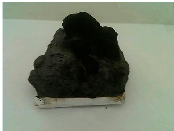
**Figure 9.** Residue of HT/E-15APP after cone calorimetry tests.
