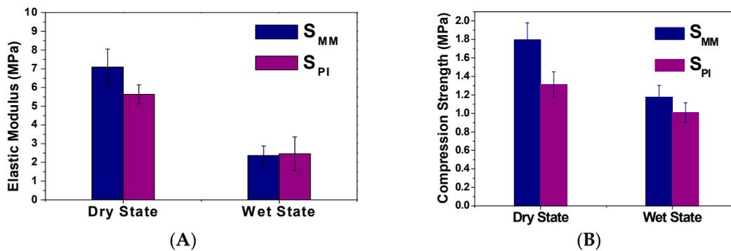
**Figure 4.** Elastic modulus (A) and compression strength (B) of  $S_{MM}$  and  $S_{PI}$  in dry and wet states.
