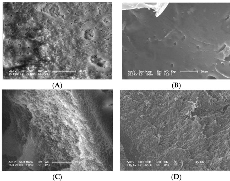
Figure 2. SEM images of pore surface and wall of  $S_{PI}$  (A,C) and  $S_{MM}$  (B,D). The bar length is 20  $\mu\text{m}$ .
