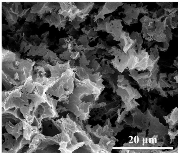
**Figure S1.** SEM image of fracture surface of scaffolds formed by P85-20.
