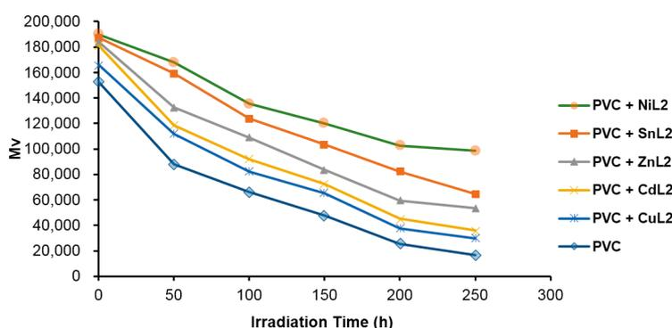
Figure 7. Effect of irradiation time (250 h) on  $\bar{M}_V$  (g/mol) for PVC films (40  $\mu\text{m}$  thickness) containing  $\text{ML}_2$  (0.5 wt %).
