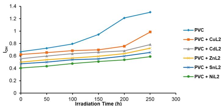
Figure 6. Effect of irradiation time (250 h) on  $I_{OH}$  and for PVC films (40  $\mu\text{m}$  thickness) containing  $\text{ML}_2$  (0.5 wt %).
