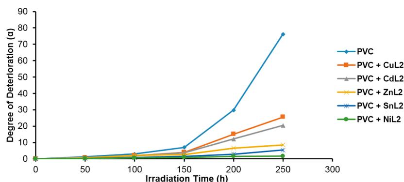
**Figure 9.** Effect of irradiation time (250 h) on  $\alpha$  for PVC films (40  $\mu\text{m}$  thickness) containing ML<sub>2</sub> (0.5 wt %).
