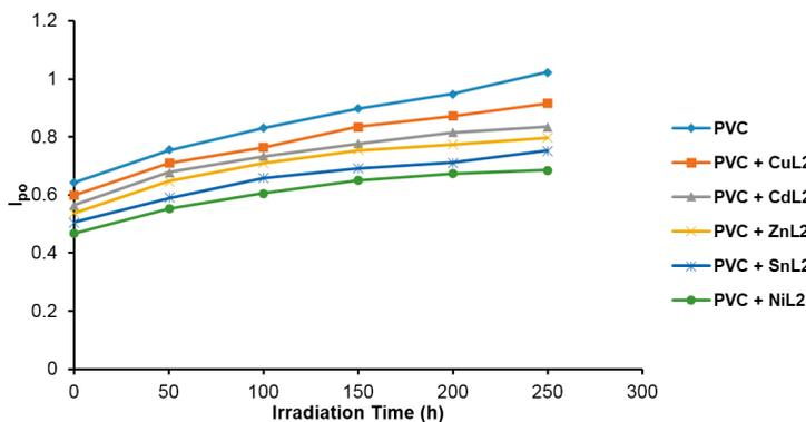
Figure 5. Effect of irradiation time (250 h) on  $I_{PO}$  and for PVC films (40  $\mu\text{m}$  thickness) containing  $\text{ML}_2$  (0.5 wt %).
