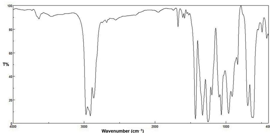
Figure 2. FTIR spectrum of poly(vinyl chloride) (PVC) film before irradiation.
