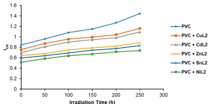
Figure 4. Effect of irradiation time (250 h) on  $I_{CO}$  for PVC films (40  $\mu\text{m}$  thickness) containing  $\text{ML}_2$  (0.5 wt %).
