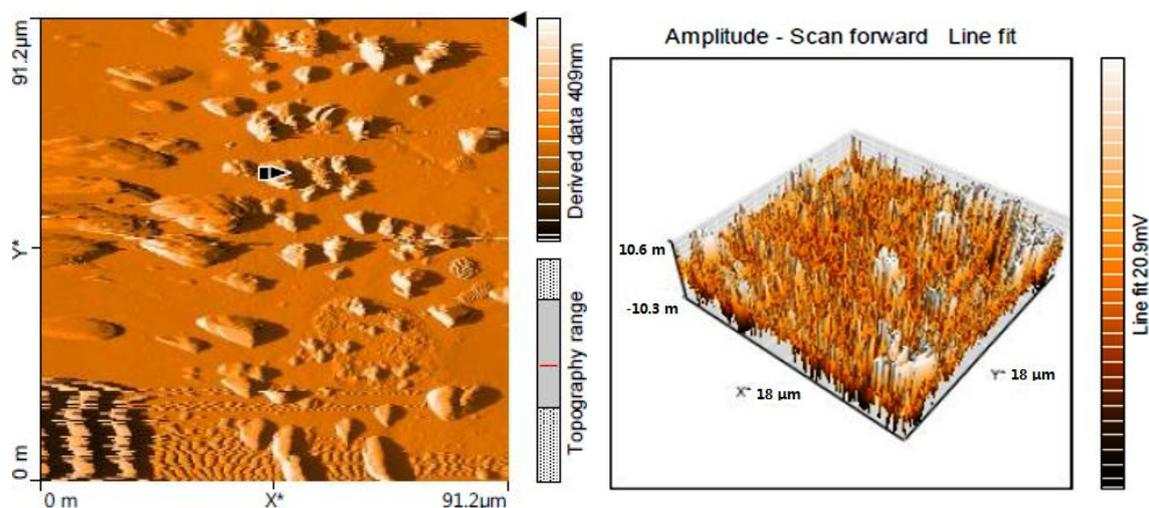
Figure 10. 2D and 3D AFM images of PVC film (control) exposed to UV light for 250 h.
