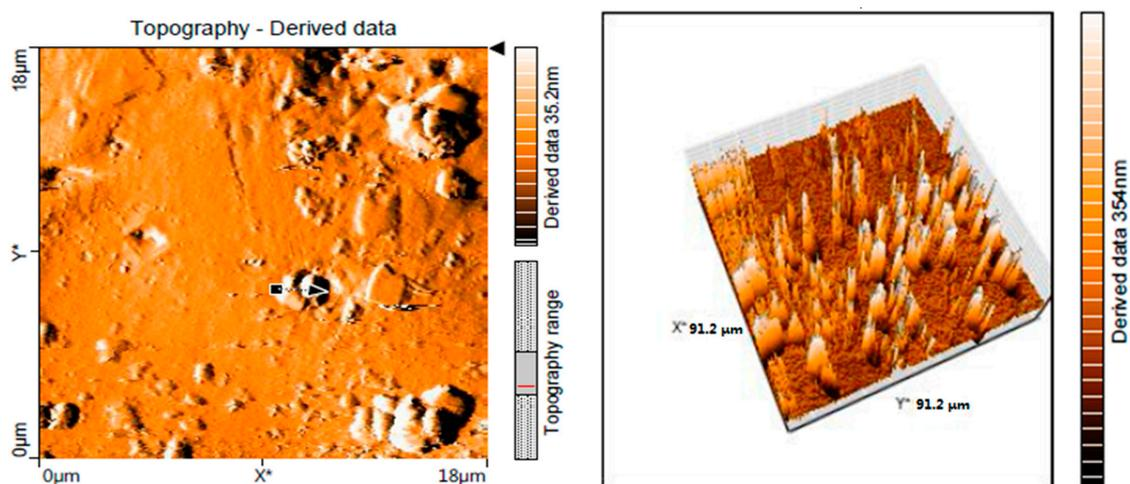
Figure 11. 2D and 3D AFM images of PVC film containing Ni(II) exposed to UV light for 250 h.
