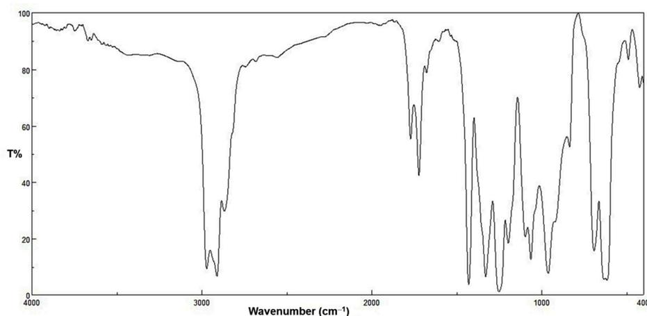
Figure 3. FTIR spectrum of PVC film after irradiation for 250 h.
