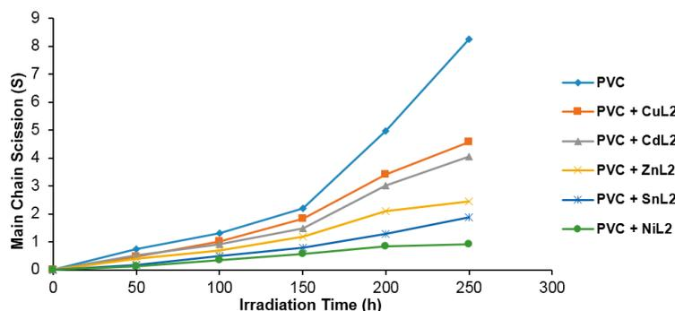
Figure 8. Effect of irradiation time (250 h) on  $S$  for PVC films (40  $\mu\text{m}$  thickness) containing  $\text{ML}_2$  (0.5 wt %).
