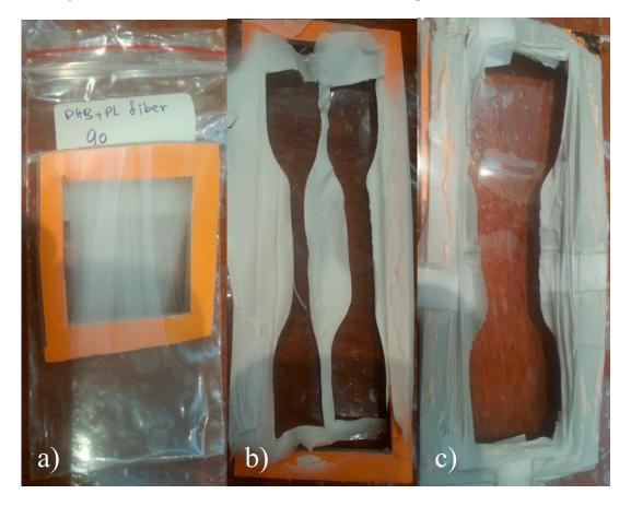
**Figure S3.** Fiber rolling after electrospinning processes on the frame and the method to collects by the frame for the dumb bell shape.
