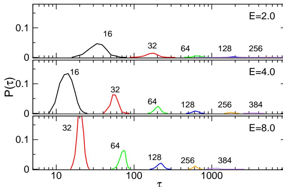
**Figure S1.** Probability distribution  $P(\tau)$  of translocation time at  $E = 2.0, 4.0,$  and  $8.0$ . The chain length  $N$  is indicated near the curves.
