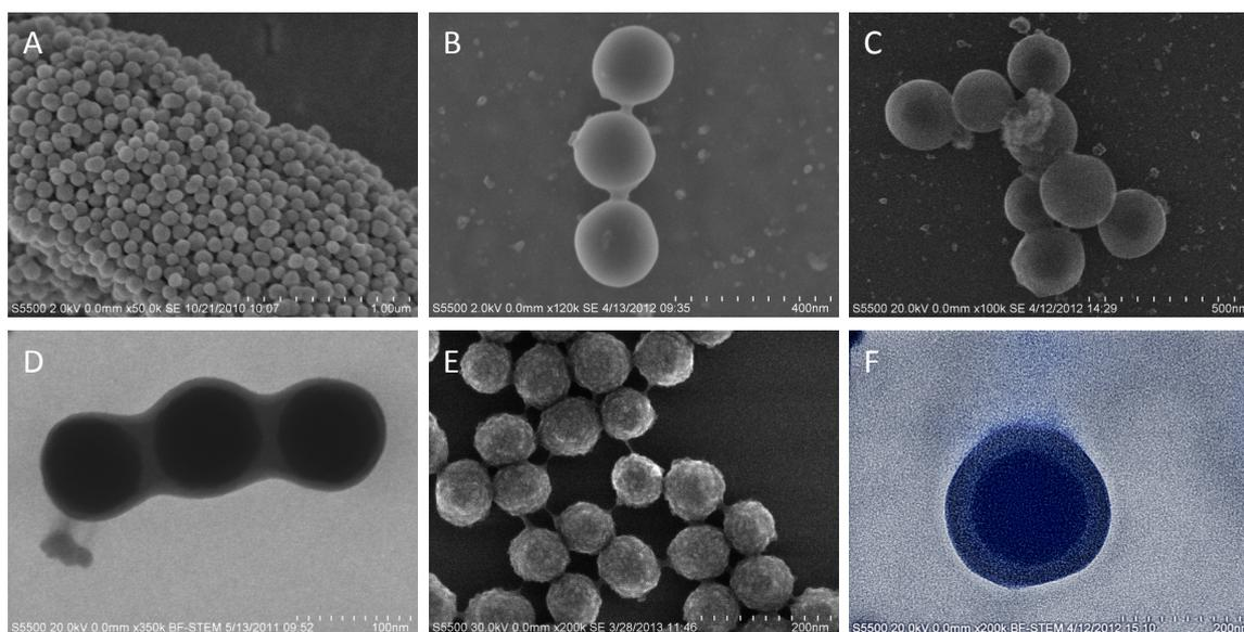
**Figure 6.** FE-SEM images of Si-NP of different size and state of decoration. (A) and (B): bare Si-NP; (C): ATRP initiator decorated NP; (D): PBMA brush decorated Si-NP; (E) and (F): PMAA brush decorated Si-NP.
