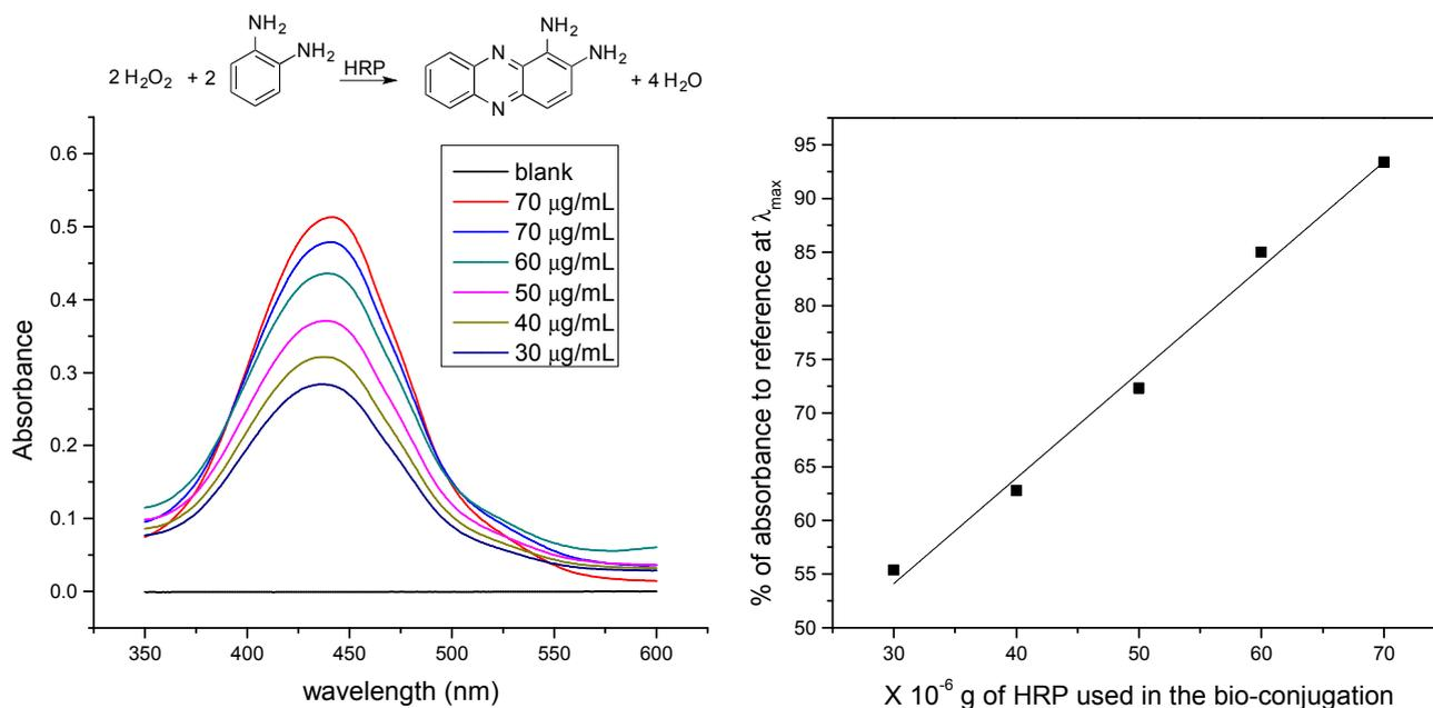
**Figure 7.** Horseradich peroxidase (HRP) catalysed conversion of *o*-phenylene diamine dihydrochloride (OPD) into 2,3-diaminophenazine and significant UV-Vis absorbance peaks of 2,3-diaminophenazine for reactions catalysed by Si-NP conjugated with HRP at a concentration of 1 mg/mL NP in PBS at pH 7.4. Experiments 1–5 represent NP with decreasing amounts of conjugated HRP. The reference sample was recorded with free HRP (70 µg/mL), while the blank contains no HRP.
