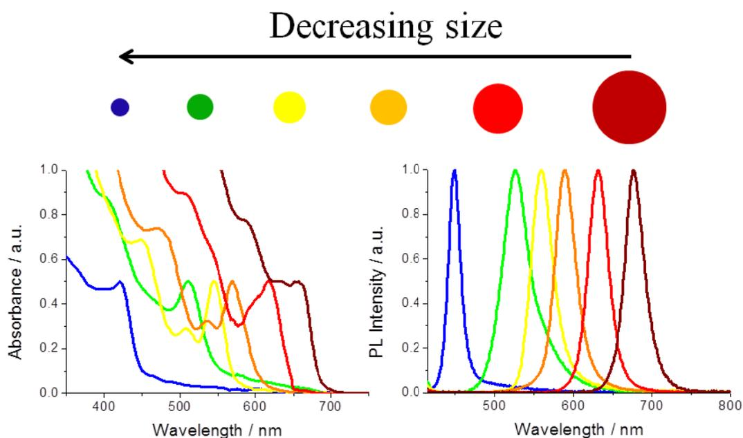
**Figure 2.** Size- and material-dependent emission spectra of several colloidal semiconductor NCs in a variety of sizes. The blue spectra represent different sizes of CdSe NCs with diameters of 2.1, 2.4, 3.1, 3.6, and 4.6 nm (from right to left). The green spectra represent InP nanocrystals with diameters of 3.0, 3.5, and 4.6 nm. The red spectra are related to InAs NCs with diameters of 2.8, 3.6, 4.6, and 6.0 nm (The image is reproduced from [12] with permission).
