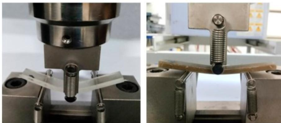
Figure 7. Flexural three-point bending test.
