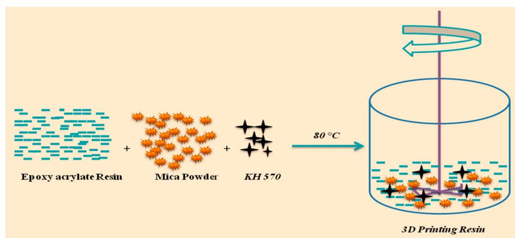
**Figure 1.** Mixing of mica and EPA resin with the addition of KH570 at 80 °C.
