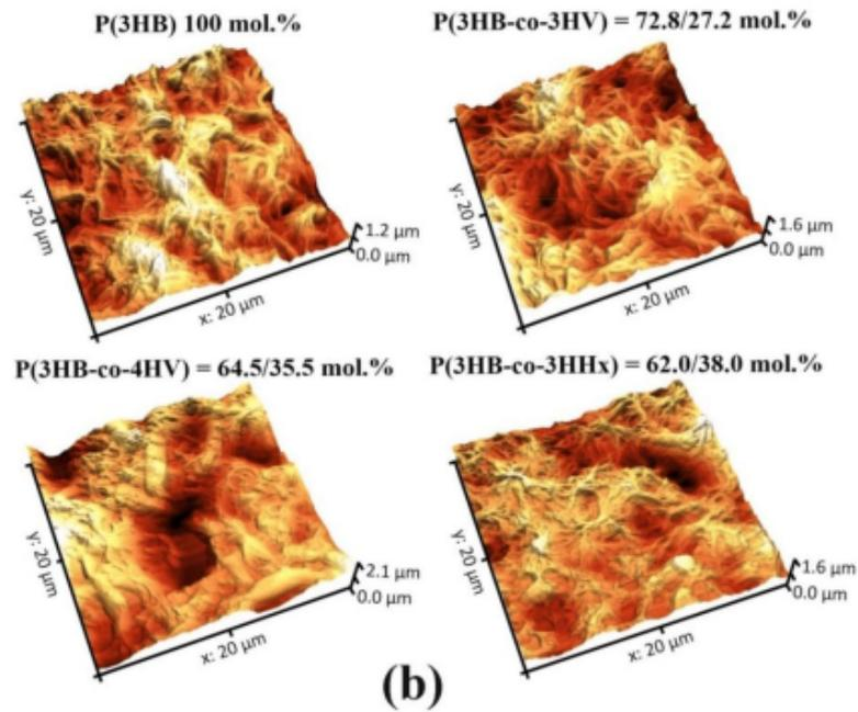
**Figure 1.** SEM (a) and AFM (b) images of pristine (non-treated) polymer films prepared from PHAs with different chemical composition.
