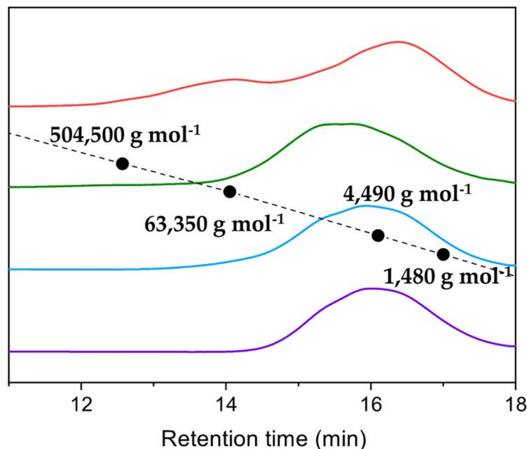
**Figure 5.** Gel permeation chromatograms of isolated polymers obtained with [WCl<sub>4</sub>(THF)<sub>2</sub>] (red), [WC<sub>14</sub>(MeCN)<sub>2</sub>] (violet), [WBr<sub>2</sub>(CO)<sub>3</sub>(dme)] (light blue) and [Mo<sub>2</sub>(CO)<sub>3</sub>(MeCN)<sub>2</sub>] (green) as catalysts.
