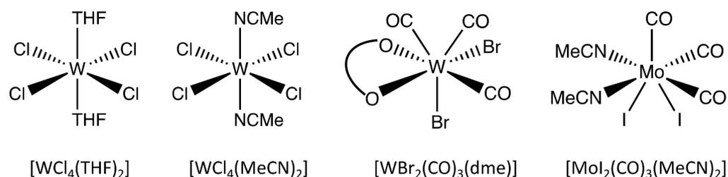
**Figure 2.** Chemical structures of the used catalysts. THF = tetrahydrofuran, MeCN = acetonitrile, dme = dimethoxyethane.
