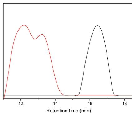
**Figure 9.** Gel permeation chromatograms of the low molar mass fraction ( $F_{\text{low}}$ , black) and high molar mass fraction ( $F_{\text{high}}$ , red) of the product obtained by the polymerization of benzyl chloride with 0.5% mol/mol BCMD catalyzed by  $[\text{WCl}_4(\text{THF})_2]$ .
