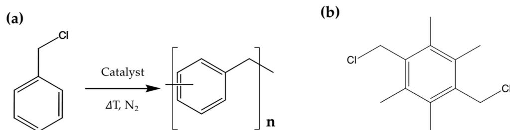
**Figure 1.** (a) Benzyl chloride polymerization scheme and chemical structure of poly(phenylene methylene). (b) Chemical structure of 1,4-bis(chloromethyl)-2,3,5,6-tetramethylbenzene (3,6-bis(chloromethyl)durene, BCMD) used as a bifunctional branching agent in this work.
