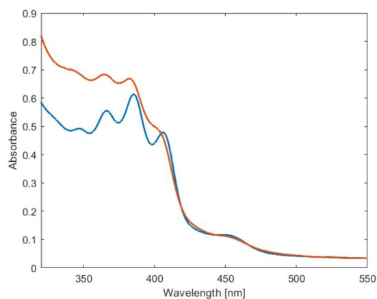
**Figure 11.** UV-vis absorption spectra of PPM (blue) and PPM-D (orange) in chloroform (0.5% m/m).
