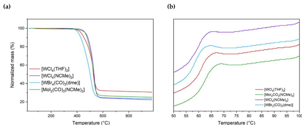
**Figure 7.** Thermogravimetric analysis (a) and differential scanning calorimetry (b) results of PPM synthesized with each catalyst.
