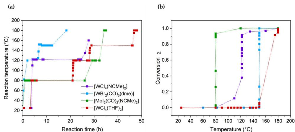
**Figure 3.** (a) Temperature ramp for each reaction catalyzed by [WCl<sub>4</sub>(MeCN)<sub>2</sub>] (violet), [WCl<sub>4</sub>(THF)<sub>2</sub>] (red), [WBr<sub>2</sub>(CO)<sub>3</sub>(dme)] (blue) and [MoI<sub>2</sub>(CO)<sub>3</sub>(MeCN)<sub>2</sub>] (green) during the heating process. (b) Monomer conversion during the polymerization reactions with each catalyst as a function of temperature.
