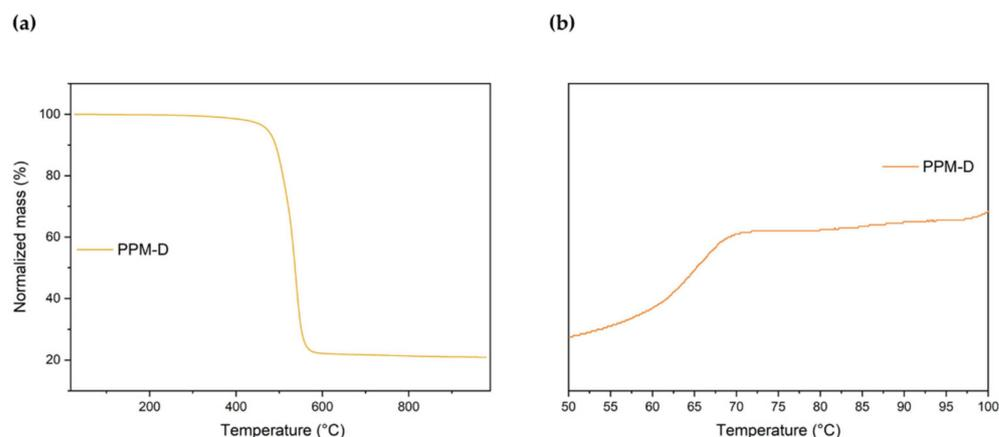
**Figure 13.** Thermogravimetric analysis (a) and differential scanning calorimetry (b) results of PPM synthesized in the presence of BCDM.
