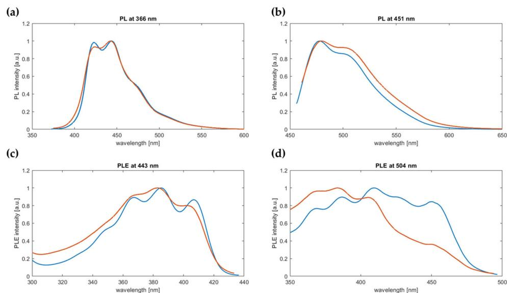
**Figure 12.** Normalized optical spectra of PPM (blue) and PPM-D (orange), both synthesized with the catalyst  $[\text{WCl}_4(\text{THF})_2]$ . Above, PL recorded upon exciting the polymer at 366 nm (a) (corresponding to the total photoluminescence emission), and at 451 nm (b) (corresponding to the green phase emission). Below, PLE spectra for emission detected at 443 nm (c) and 504 nm (d).
