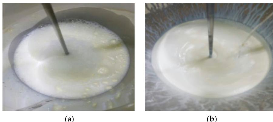
**Figure 12.** Photograph of ceria slurry before (a) and after the addition of the G-336 defoaming polymer (b).
